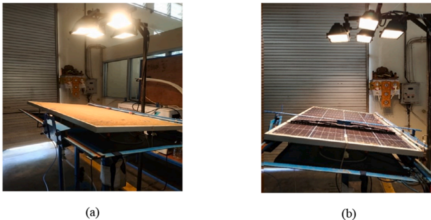
Fig. 8. Experimental setup for self-cleaning with (a) dusty surface and (b) clean surface [72].
