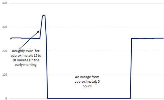
Fig. 3. Line-to-line voltage measurements on the X-Y connected transformer.
