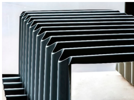
Figure 4. Bent corrugated sheet.
