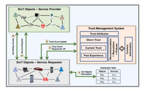
Fig. 6. High-level overview of trustworthiness management system in service-oriented SIoT.
