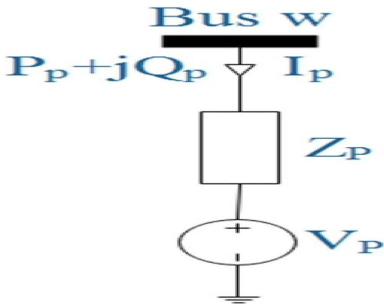
Fig. 15 STATCOM equivalent circuit
