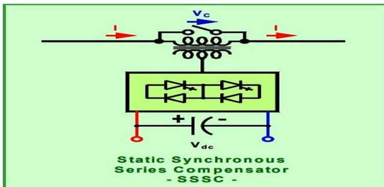
Fig. 16 SSSC schematic diagram
