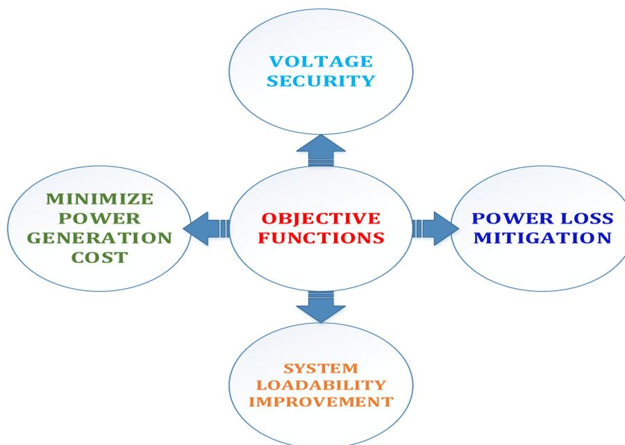
**Fig. 1** Objective functions of FACTS devices
