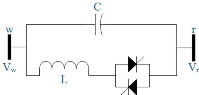
Fig. 10 T.C.S.C schematic diagram
