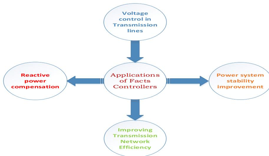
**Fig. 4** FACTS controllers applications in power systems
