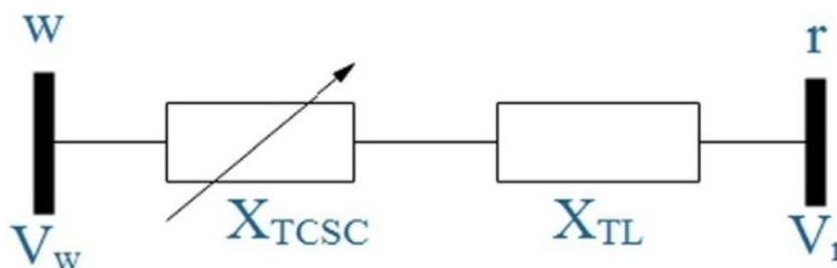
**Fig. 11** T.C.S.C equivalent diagram
