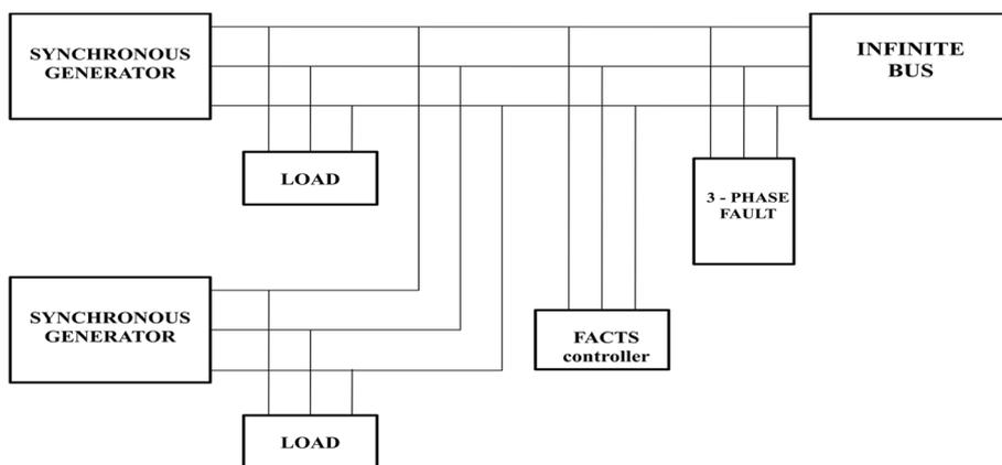
**Fig. 7** Block diagram for power system with FACTS devices
