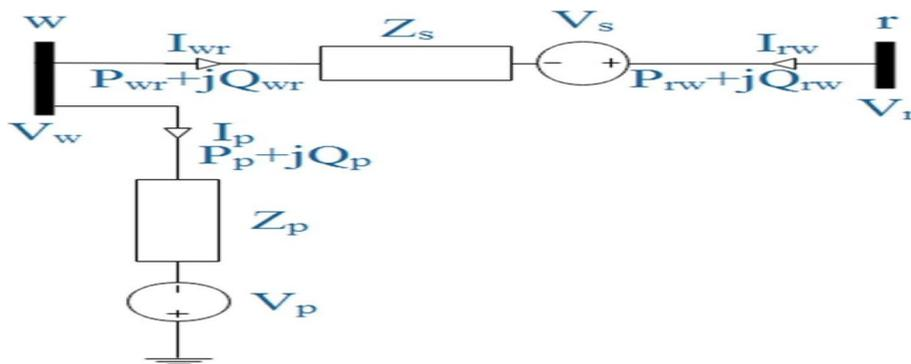
Fig. 9 UPFC equivalent diagram
