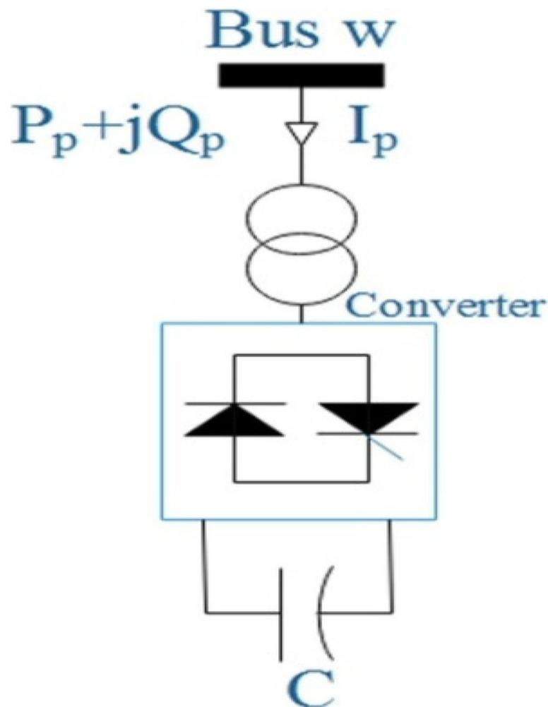
**Fig. 14** STATCOM schematic diagram
