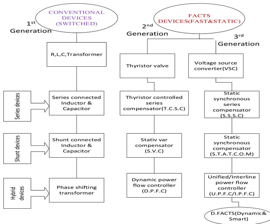
**Fig. 5** Diagram for conventional devices and FACTS devices
