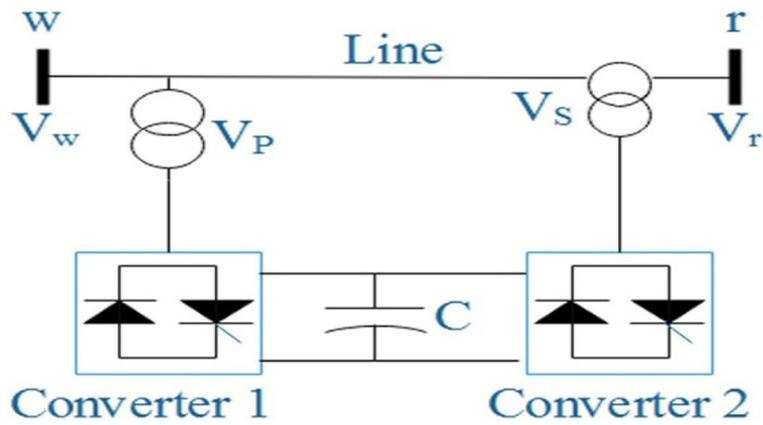
Fig. 8 UPFC equivalent diagram
