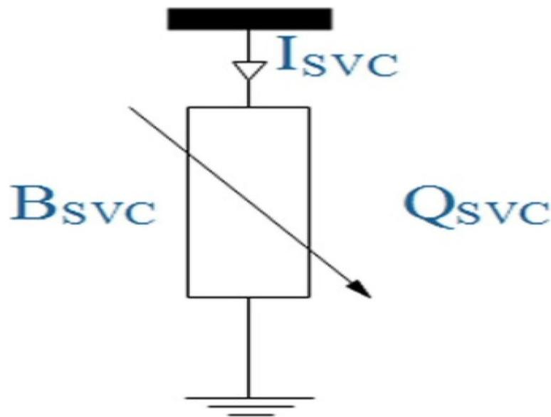
**Fig. 13** SVC equivalent circuit
