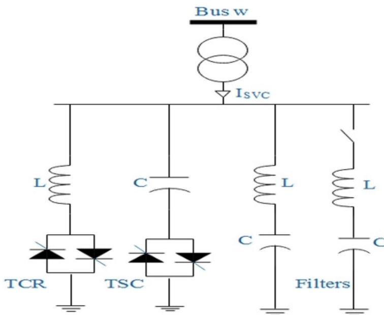
**Fig. 12** SVC schematic diagram
