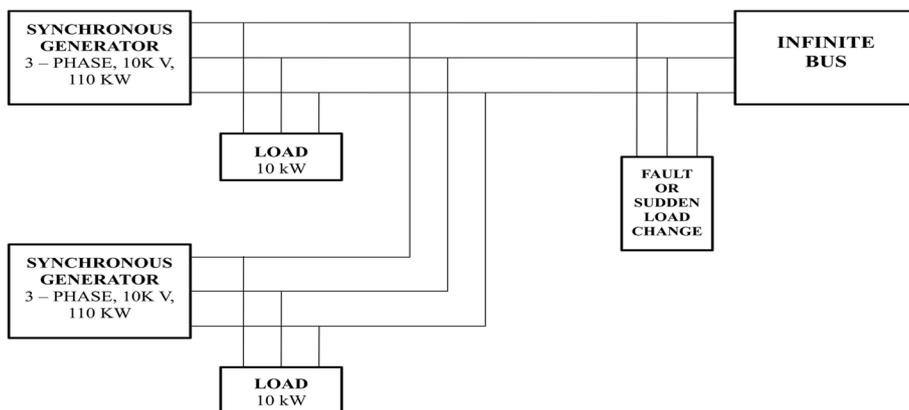
**Fig. 6** Block diagram for power system without FACTS devices
