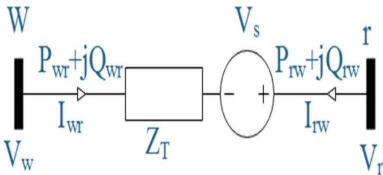
Fig. 17 SSSC equivalent circuit
