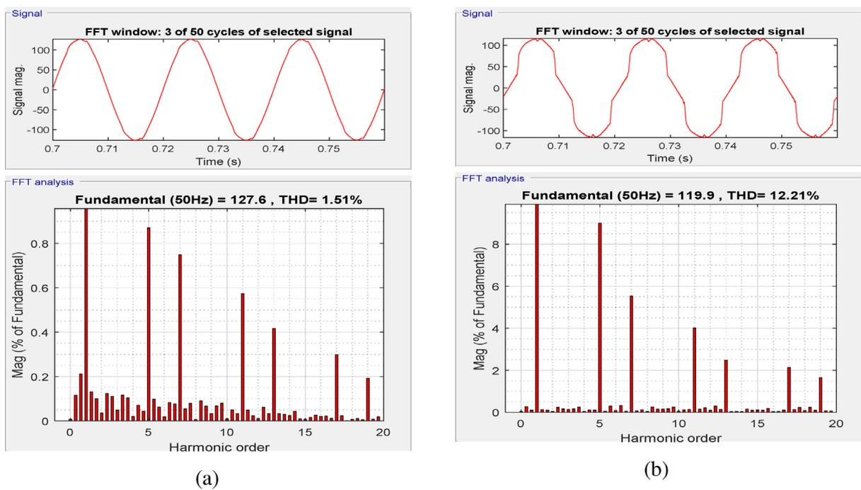
Fig. 17. THD spectrum of, (a) source current, (b) load current.
