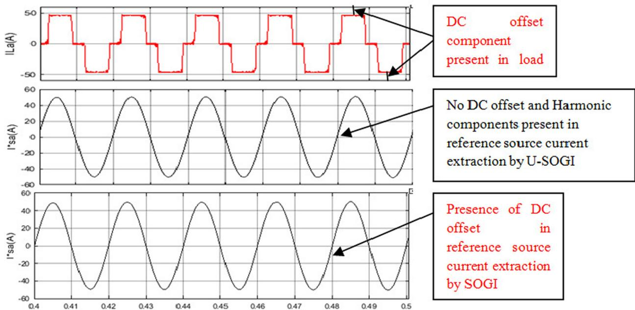
Fig. 11c. Shows the DC offsets removal capability of U-SOGI over the SOGI (x-axis in sec).
