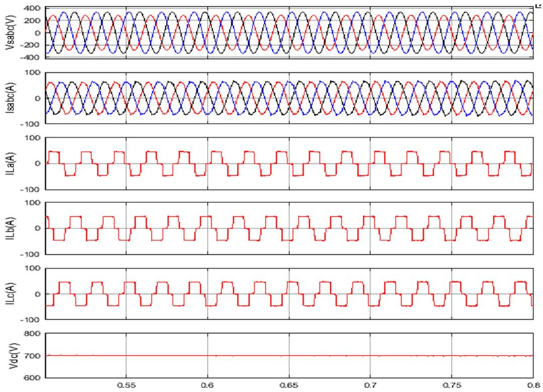
Fig. 12c. Performance of DSTATCOM under unbalanced grid voltage with U-SOGI controller (x-axis in sec).
