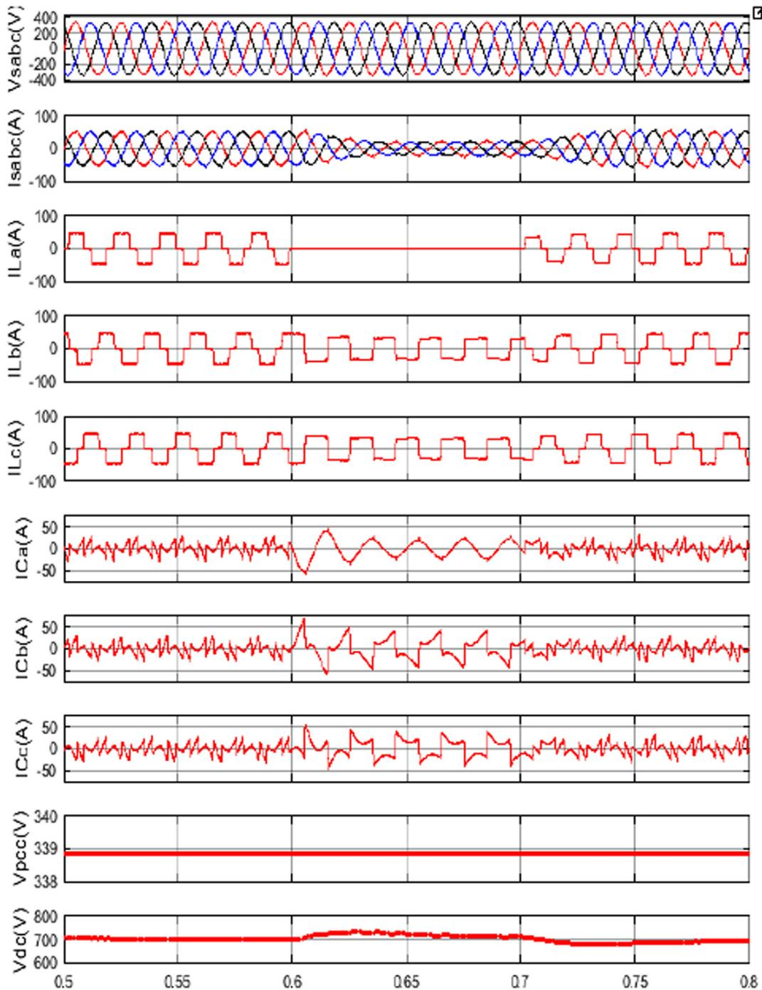
Fig. 8. ZVR mode DSTATCOM performances with nonlinear load (x-axis in sec).
