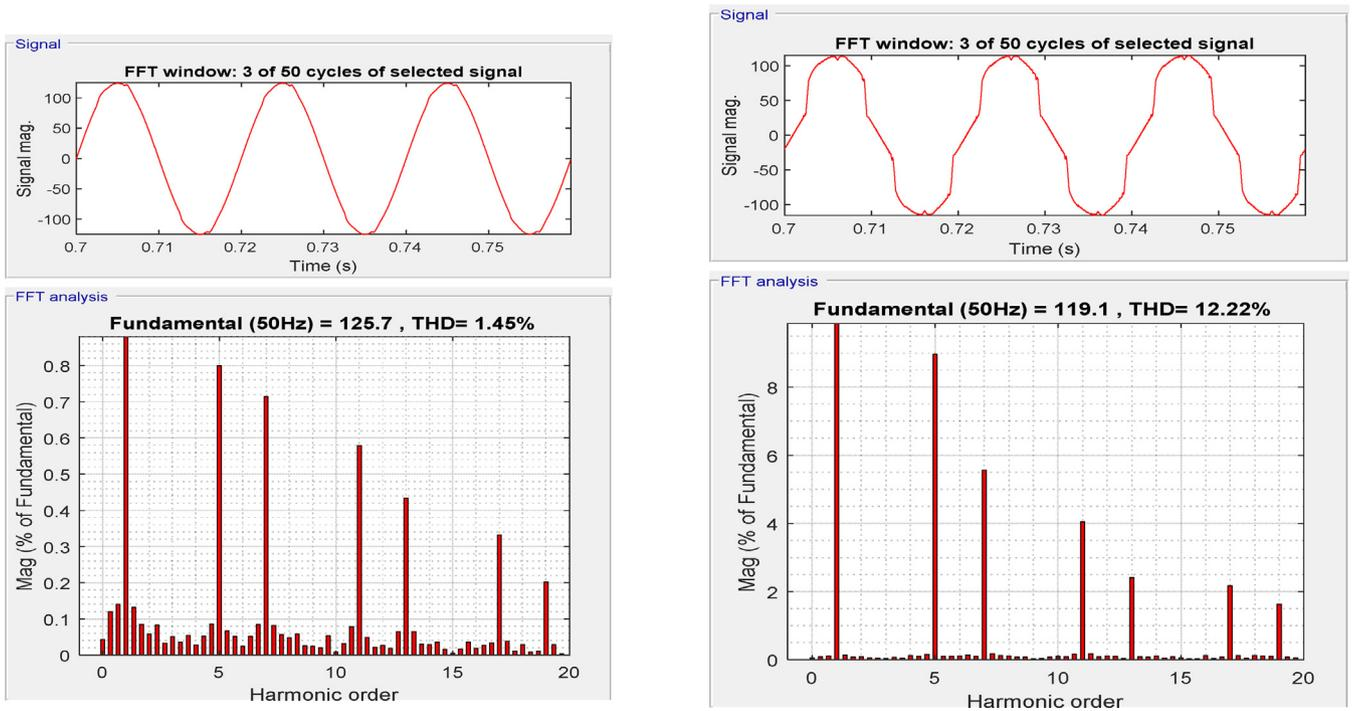
Fig. 15. THD spectrum of, (a) source current, (b) load current.
