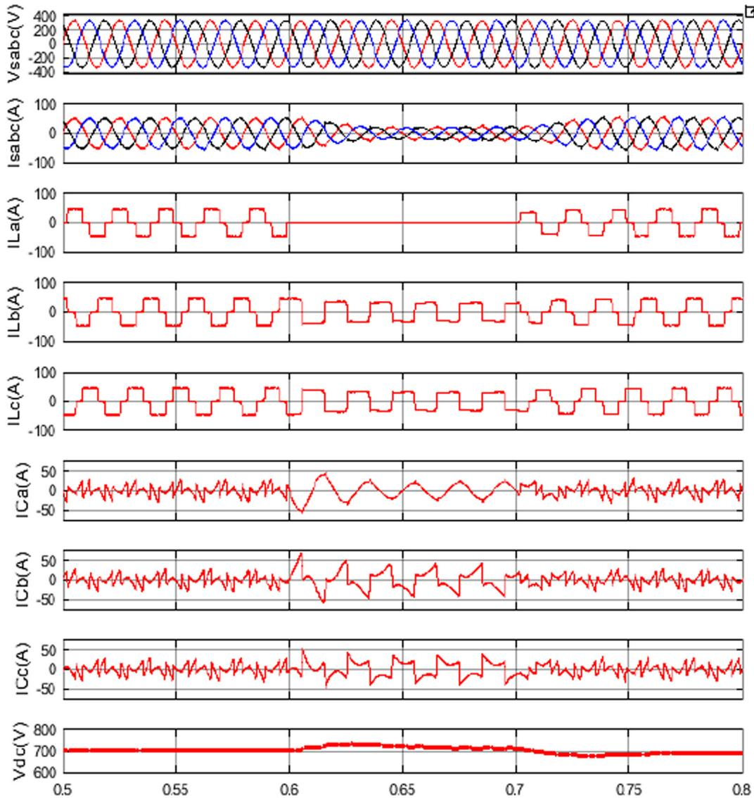
Fig. 4. PFC mode DSTATCOM performances with nonlinear load (x-axis in sec).
