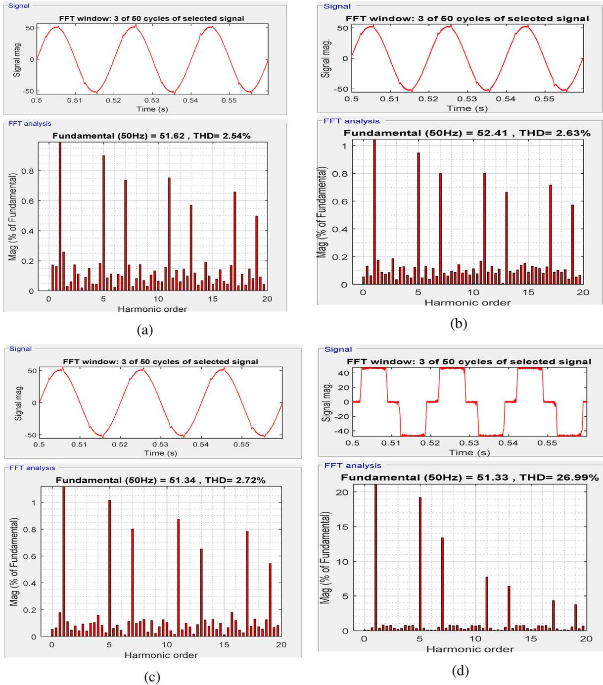
**Fig. 5.** In PFC mode THD spectrum with nonlinear load, (a) source current with proposed controller, (b) source current with ISOGI controller, (c) source current with SOGI controller,(d) load current.
