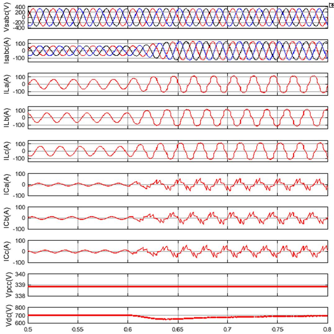
Fig. 16. Robustness of proposed controller with DSTATCOM in ZVR mode (x-axis in sec).
