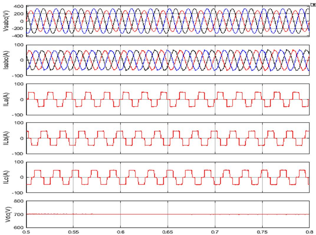
Fig. 12b. Performance of DSTATCOM under unbalanced grid voltage with ISOGI controller (x-axis in sec).
