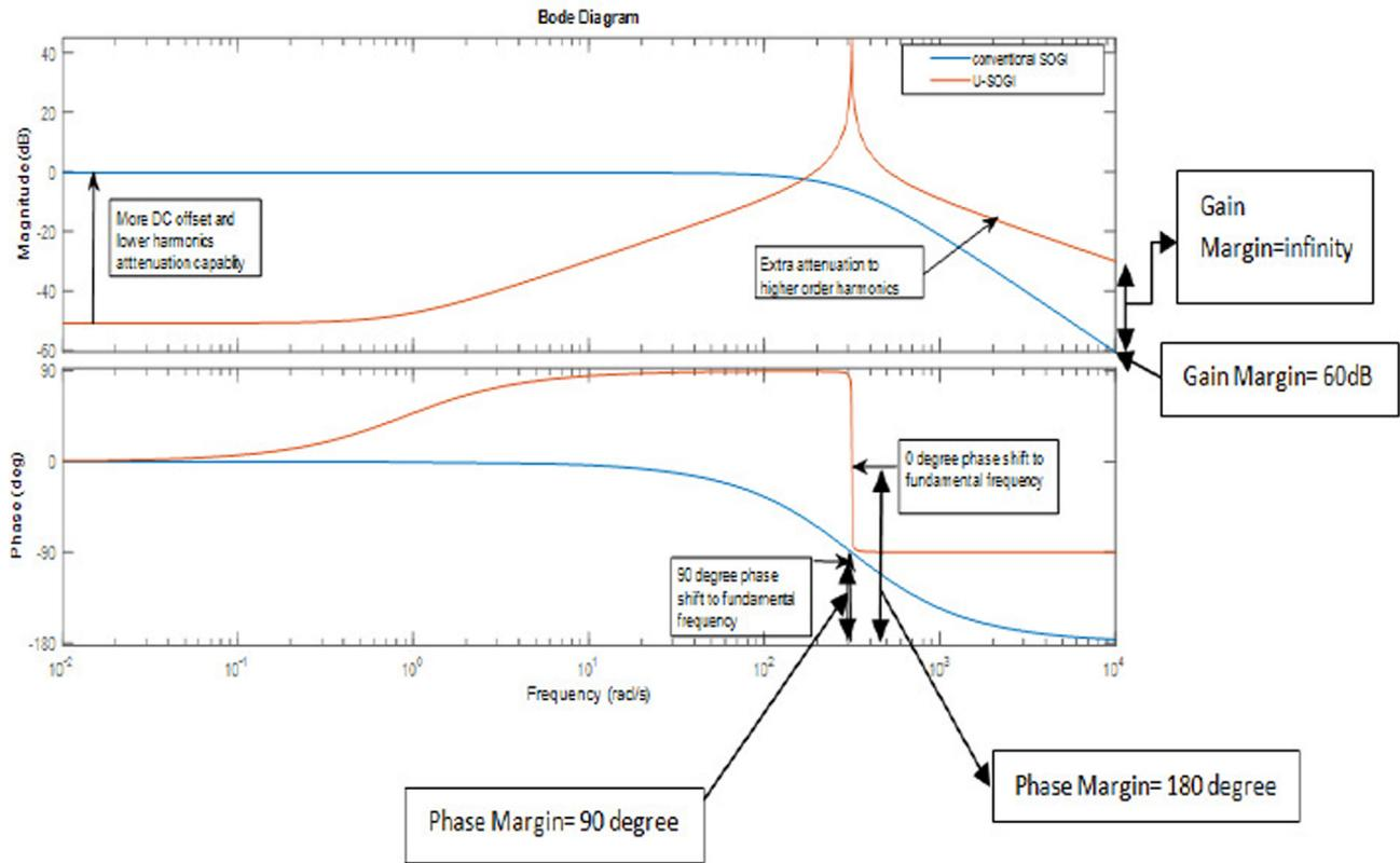
Fig. 11b. Bode plot for SOGI and U-SOGI controller.
