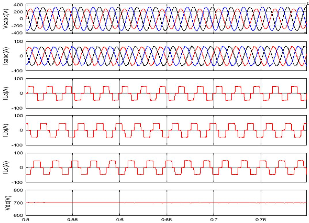
Fig. 12a. Performance of DSTATCOM under unbalanced grid voltage with SOGI controller (x-axis in sec).
