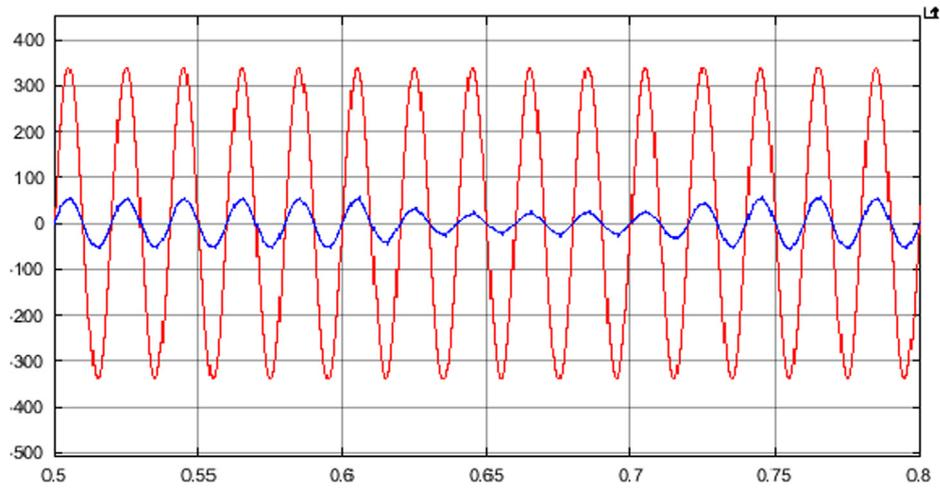
Fig. 10. Waveforms source voltage and source current (x-axis in sec).
