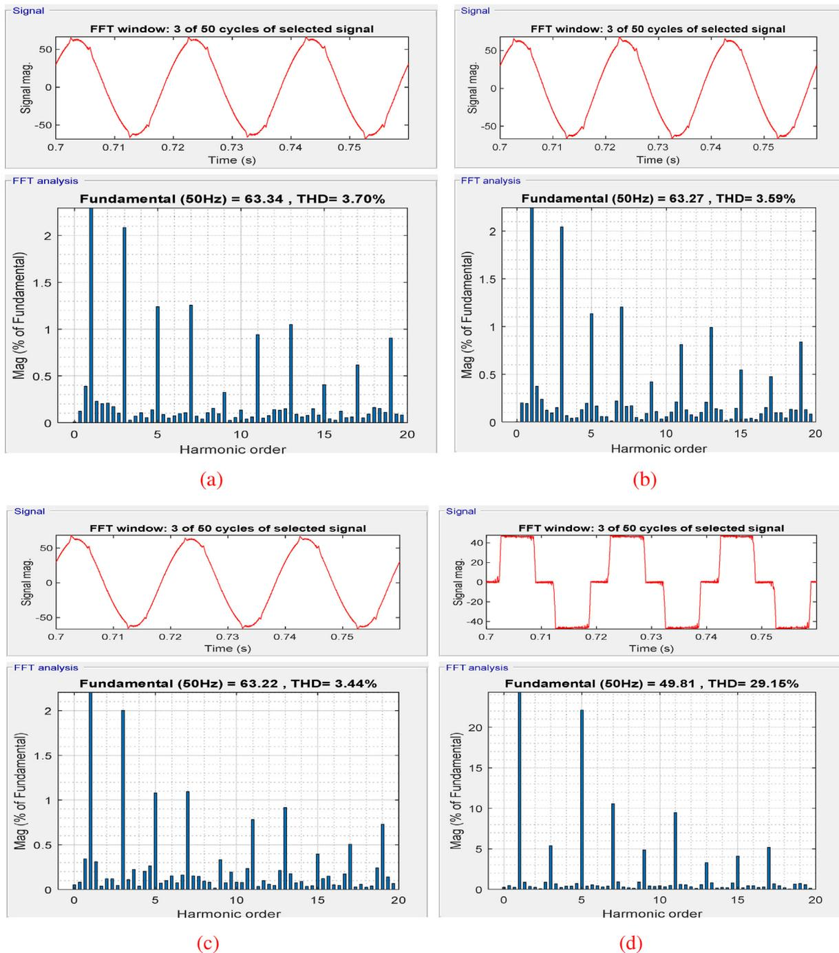
Fig. 13. Source current THD spectrum with (a) SOGI, (b) I-SOGI, (c) U-SOGI controller and (d) load current THD spectrum.
