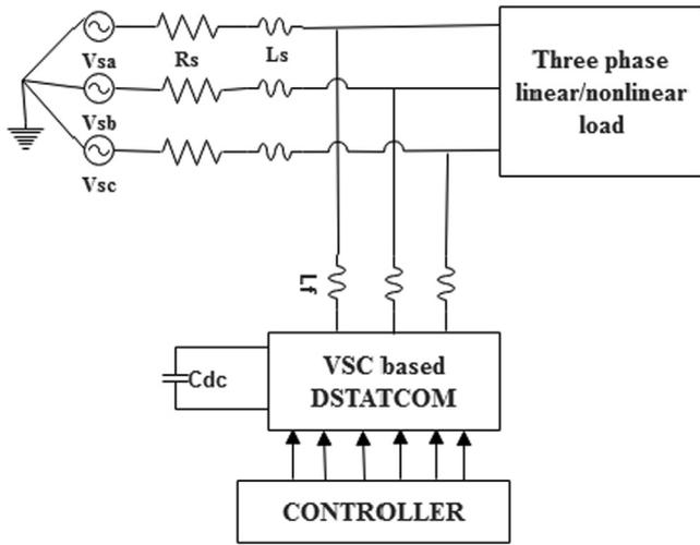
Fig. 1. DSTATCOM in proposed system.
