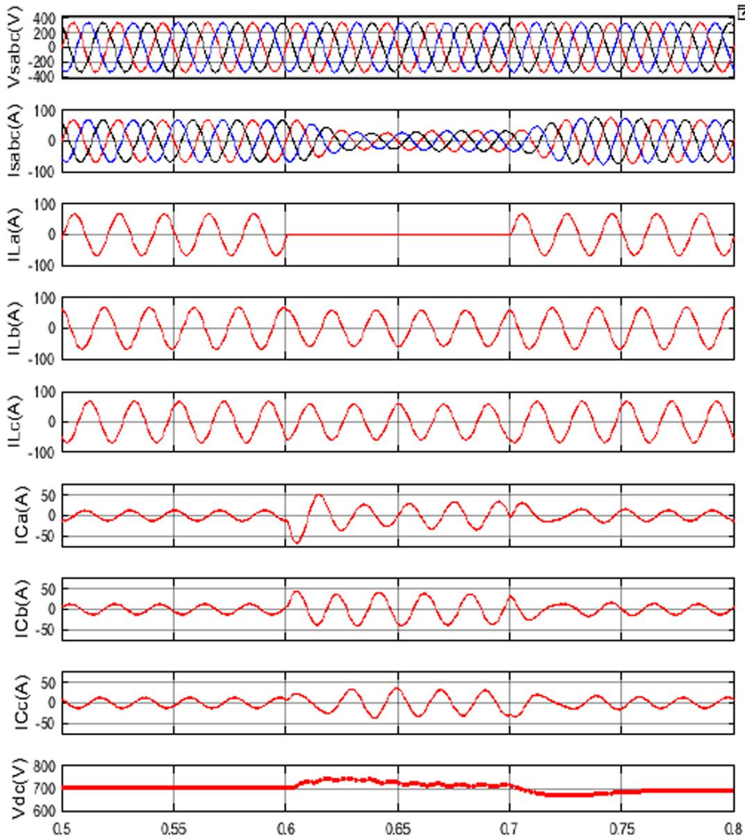
Fig. 3. PFC mode DSTATCOM performances with linear load (x-axis in sec).
