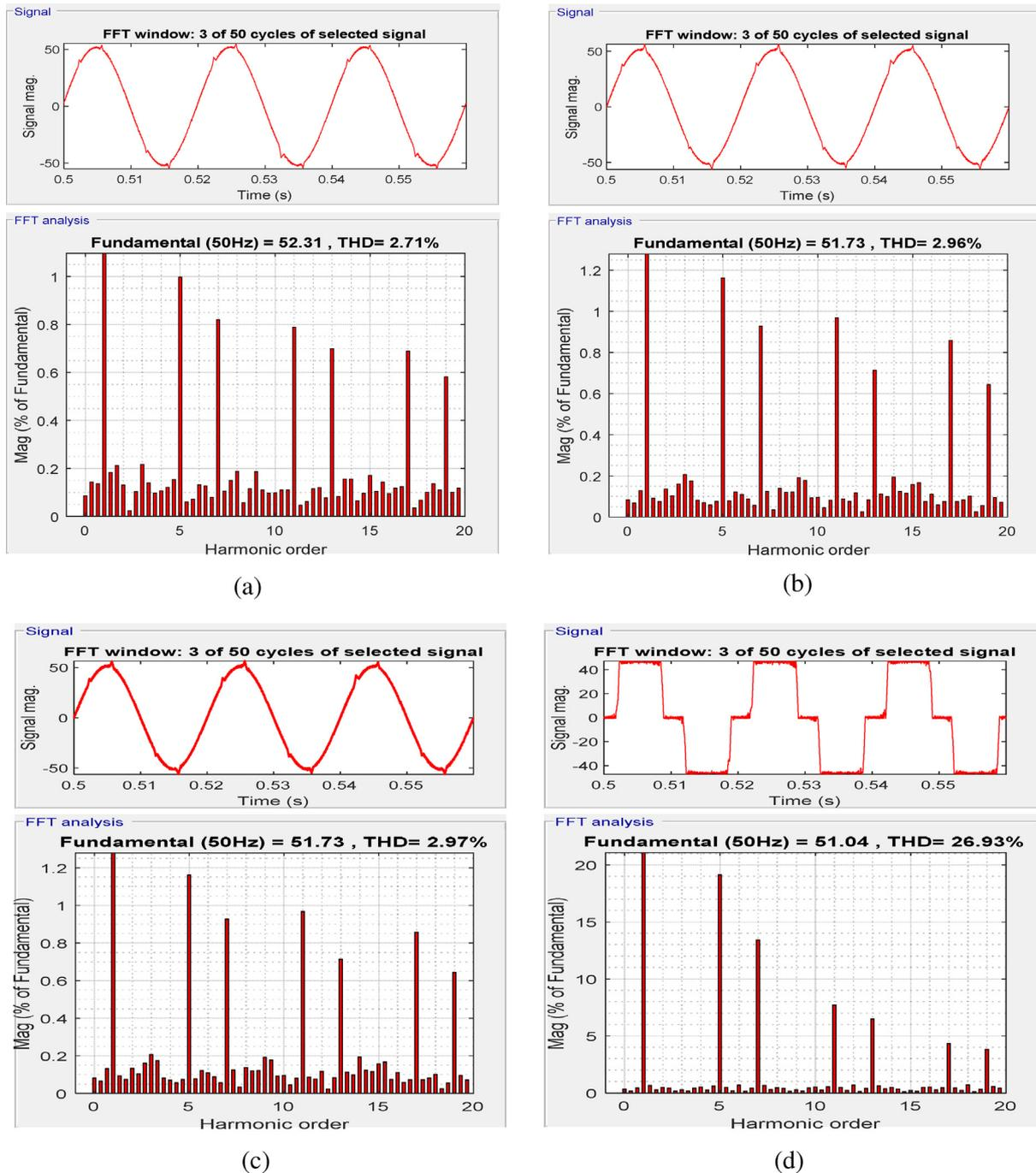
**Fig. 9.** In ZVR mode THD spectrum with nonlinear load, (a) source current with proposed controller, (b) source current with ISOGI controller, (c) source current with SOGI controller, (d) load current.
