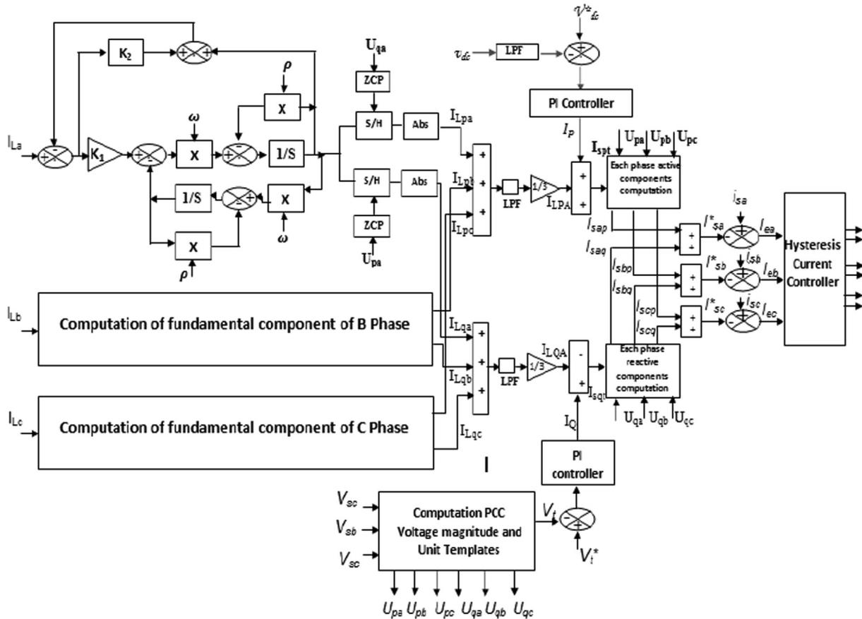
Fig. 2. Computation of reference current with U-SOGI technique.
