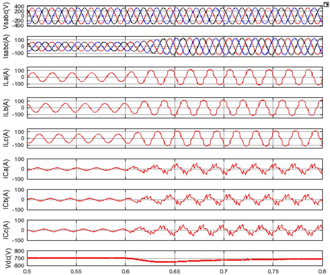
Fig. 14. Robustness of controller with DSTATCOM in PFC mode (x-axis in sec).
