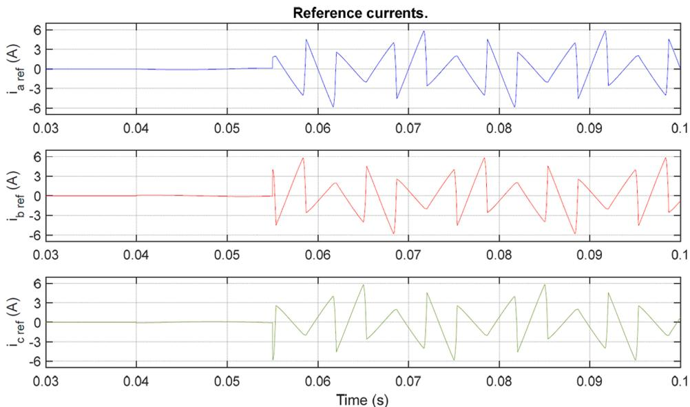
Fig. 12. SAPF compensating/reference currents waveforms. Compensation starts at  $t = 0.055$  s.
