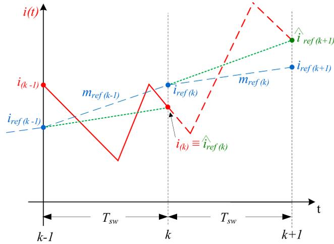
Fig. 7. Prediction of current reference value.  $i_{ref}(k+1)$ .
