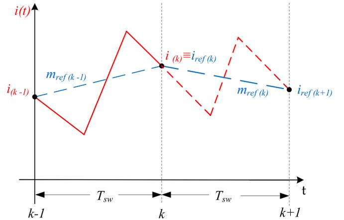
Fig. 6. Known reference value  $i_{ref(k+1)}$  in steady state.
