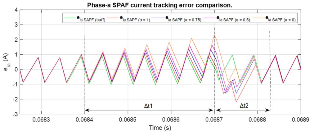
Fig. 18. Phase-a current error for: buffer case (green), full-slope case (red), weighted-slope case with  $\alpha = 0.75$  (blue), weighted-slope with  $\alpha = 0.5$  (magenta) and constant reference with  $\alpha = 0$  (orange). (For interpretation of the references to colour in this figure legend, the reader is referred to the web version of this article.)
