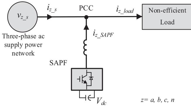
Fig. 1. Block diagram of the SAPF connection.
