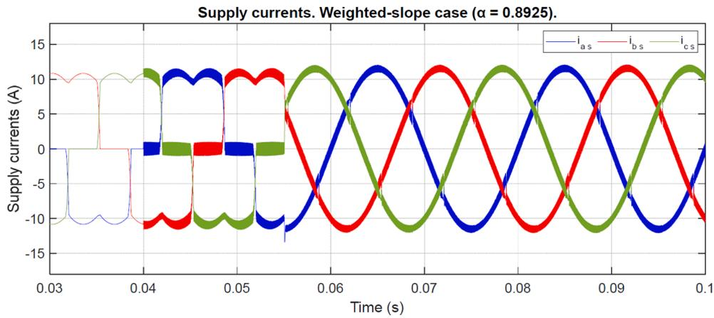
Fig. 21. Supply currents to slope weighting factor  $\alpha = 0.8925$ .
