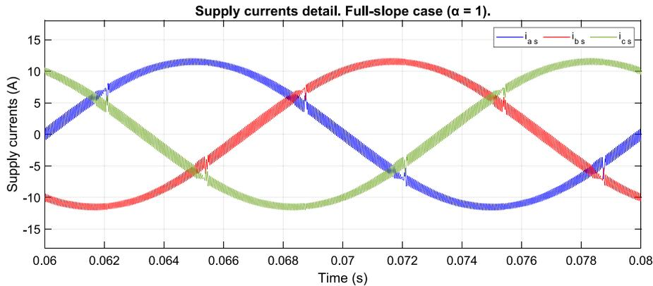
Fig. 23. Detail of supply currents to full-slope case.
