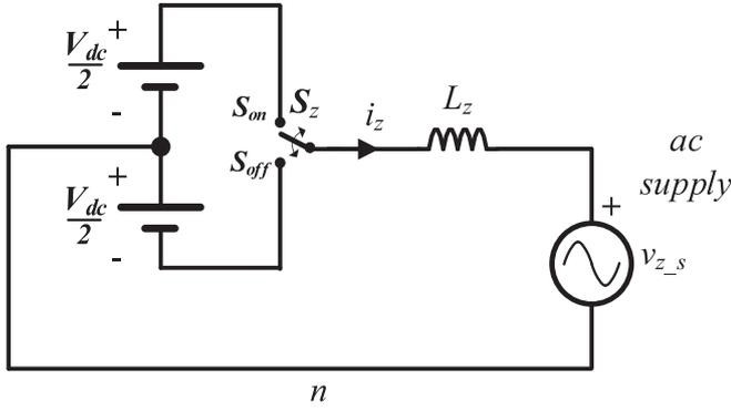
Fig. 3. Per-phase equivalent circuit of the SAPF.
