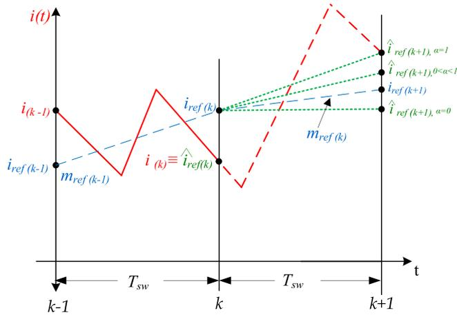
Fig. 8. Weighted-slope prediction of current reference value.  $i_{ref}(k+1)$ .
