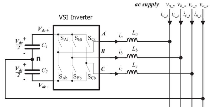
Fig. 2. Block diagram of a three-leg four-wire SAPF.
