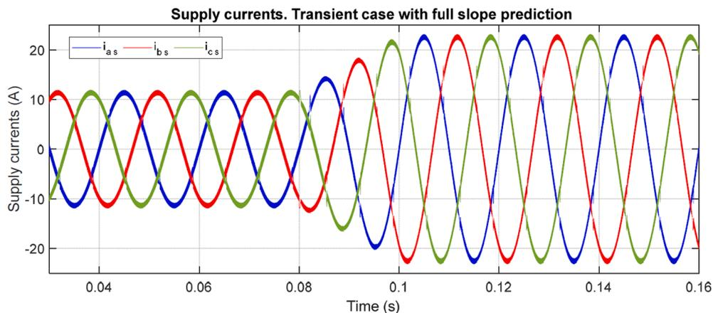
Fig. 27. Supply currents to transient with full-slope case.
