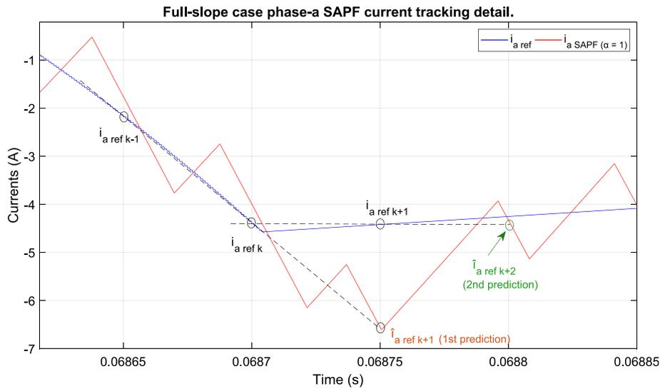
Fig. 17. Full-slope tracking when reference sign change.
