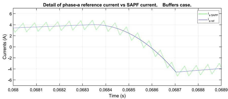
Fig. 14. Detail of the current tracking of phase-a.
