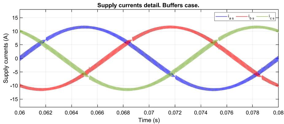
Fig. 22. Detail of supply currents to buffer case.
