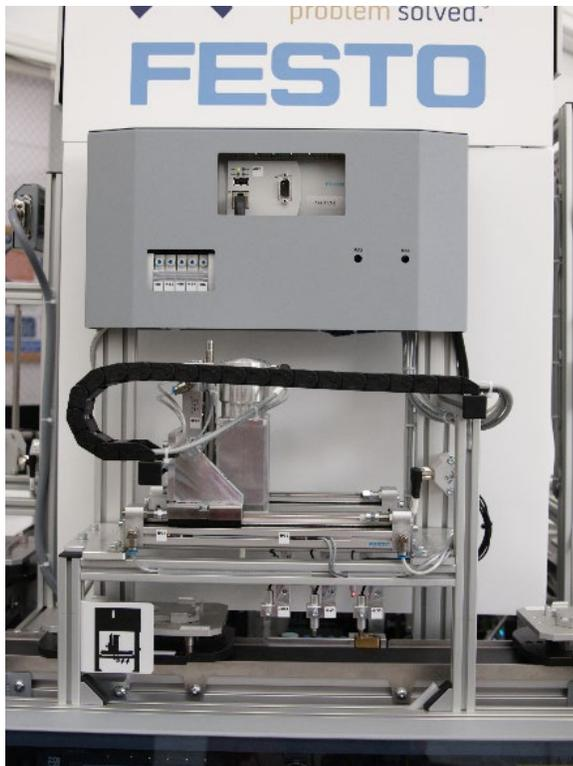
Figure 2.5: FCPL drilling module.
