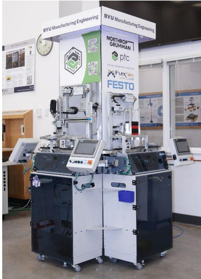
Figure 2.1: Festo Cyber-Physical Lab, showing the output module (left) and the magazine module (right).
