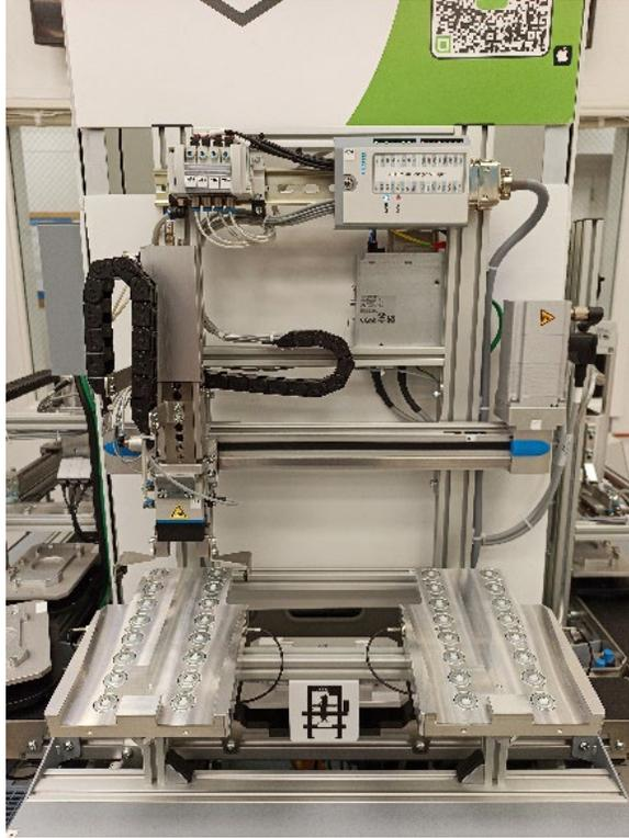
Figure 2.6: FCPL output module with the gripper over the good part tray.
