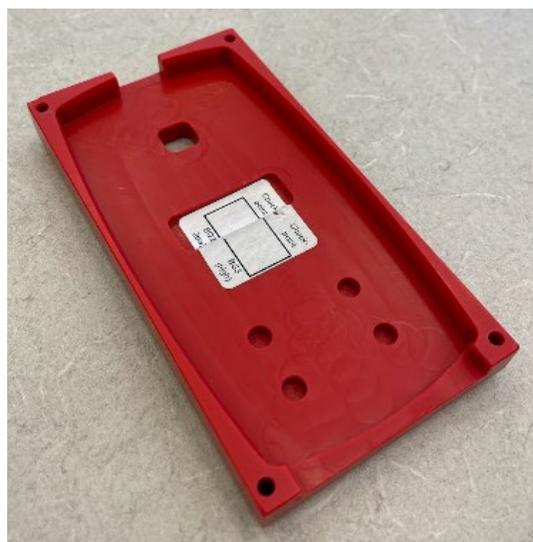
Figure 2.2: FCPL workpiece, the front cover of a simplified mobile device.
