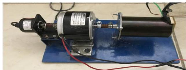
**Fig. 5.** a) Block diagram of experimental setup of the BLDC motor drive system b) Experimental setup of the BLDC motor drive system c) BLDC motor connected to DC generator as a load torque.
