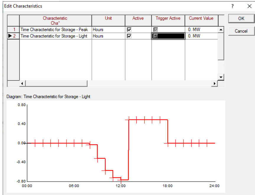
Figure 7. Absorption-Generation curve of the storage at low-load period.
