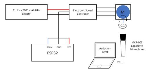
Fig. 1. Experimental setup for data acquisition.
