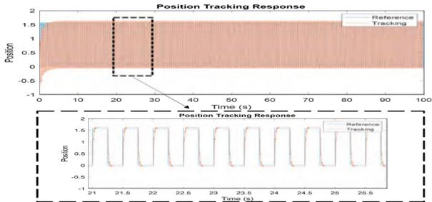
Fig. 6. Backstepping controller design response after optimization with SLDO. Top - from 0 to 100s, bottom - from 25 to 30s
