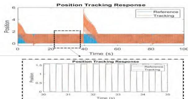
Fig. 2. Backstepping controller design response before optimization. Top - from 0 to 100s, bottom - from 30 to 35s
