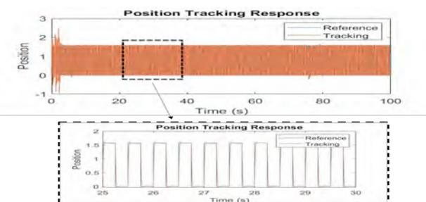
Fig. 3. Backstepping controller design response after optimization. Top - from 0 to 100s, bottom - from 30 to 35s
