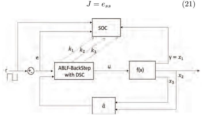
Fig. 1. Self-Optimizing Control Architecture for Brushless DC motor system
