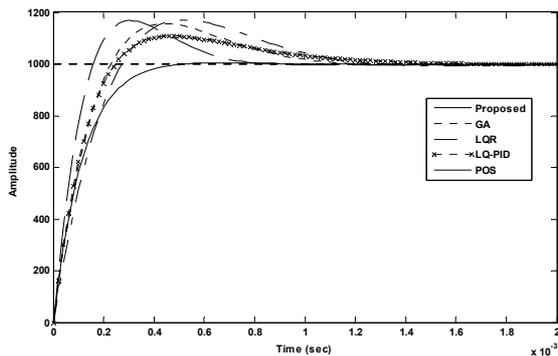
Fig. 5. Comparison between CS, LQR, LQ-pole placement, PSO and GA based PID control in speed control of BLDC motor
