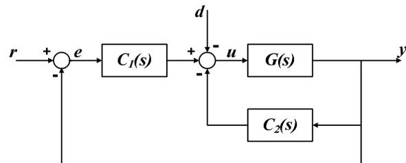
Fig. 1. Structure of Enhanced PID Control System
