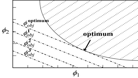
Fig. 3. Lines of constant objective functional and the region of the achievable performances.
