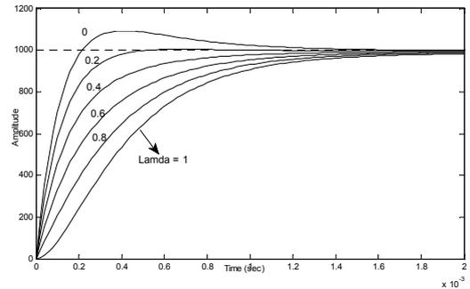
Fig. 4. According to changes, step responses of BLDC motor in CS-based PID-PD control system
