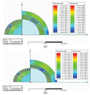
Fig. 4. The flux and current densities in a) 2.5 MW and b) 1.25 MW DFIGs
