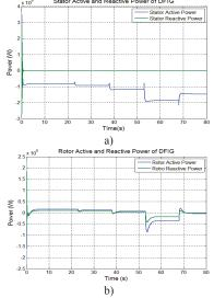
Fig. 11. The DFIG a) stator active and reactive power and b) rotor active and reactive power.
