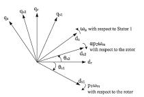
Fig. 6. Vector diagram of CDFIM reference frames.
