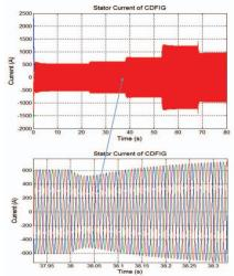
Fig. 13. The power machine stator current of CDFIG
