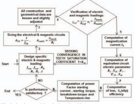
Fig. 3. The induction machine design algorithm
