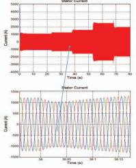
Fig. 9. The DFIG stator output current
