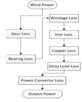
Fig. 2. Losses in WECS with DFIG
