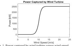
Fig. 1. Power captured by wind turbine versus wind speed.
