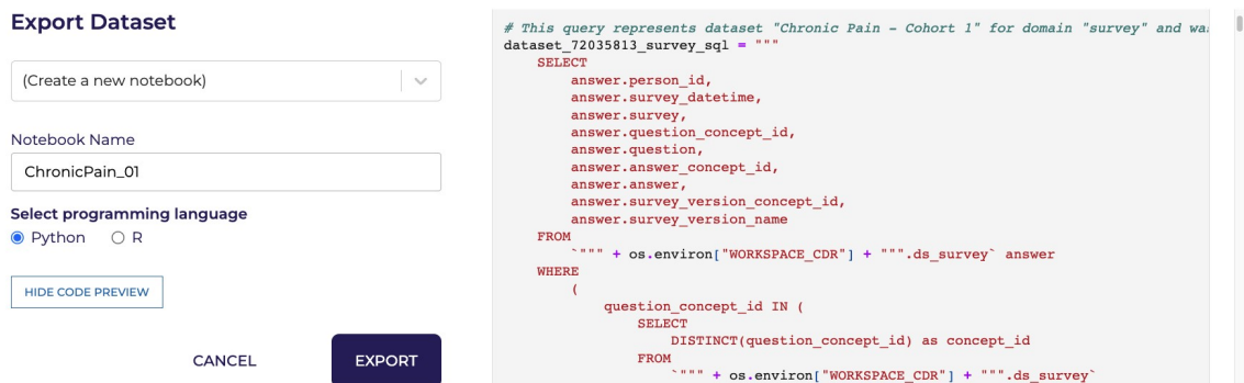
Figure 23 - Screenshot representing a preview of the SQL query prior to exporting the dataset.
