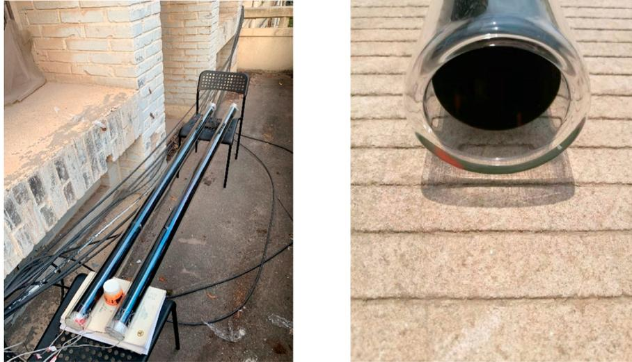
Fig. 1. All-glass straight through solar vacuum tube.
