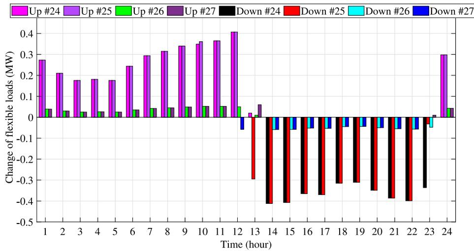
Fig. 24. Changes of flexible loads in case V.
