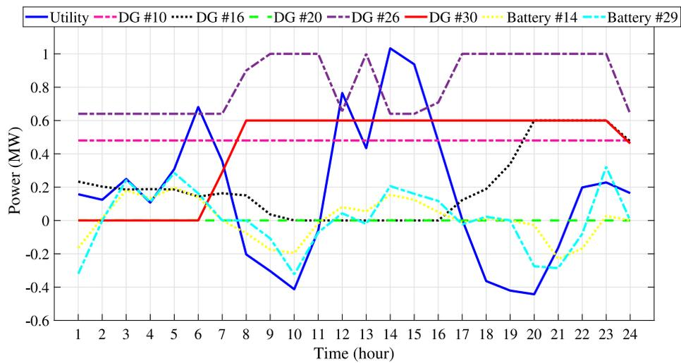
Fig. 4. Optimal DG output in case I.
