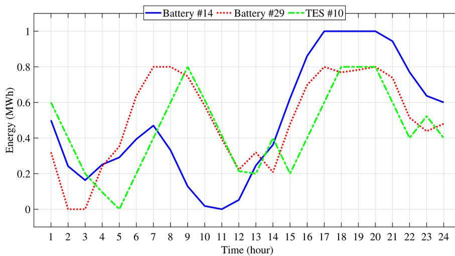
Fig. 10. Optimal energy level of energy storage devices in case II.
