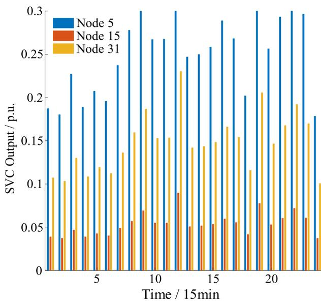
Fig. 10. SVC output after the trip out of the branch between Node 1 and 2.
