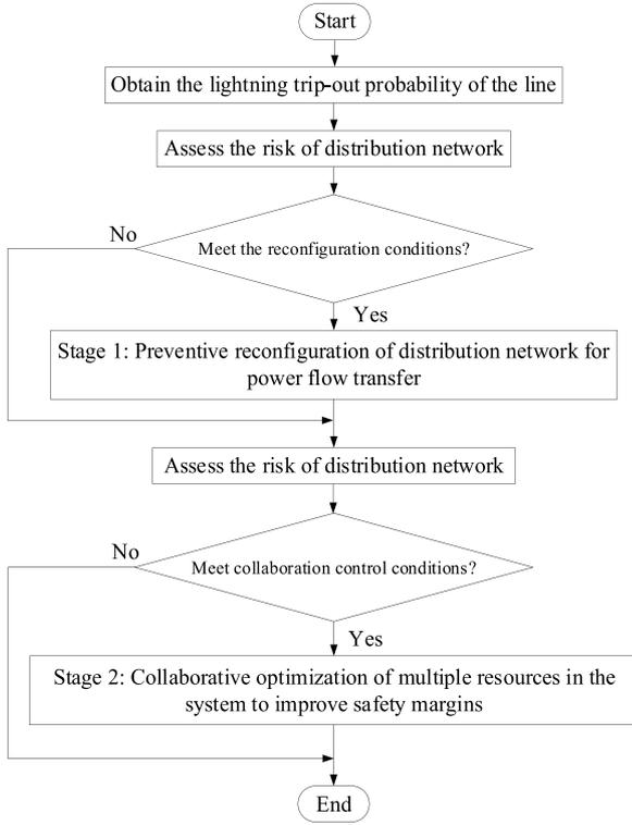
Fig. 2. Overall flow of the active lightning protection of distribution networks.
