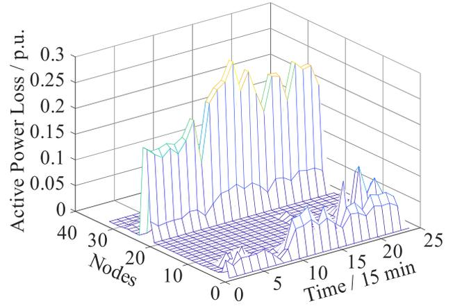
**Fig. 8.** The expected active load loss due to the accident between Node 1 and Node 2.
