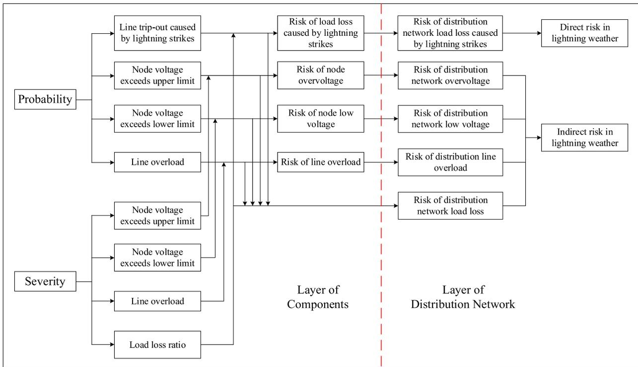
Fig. 1. The risk index system of distribution networks in lightning weather.
