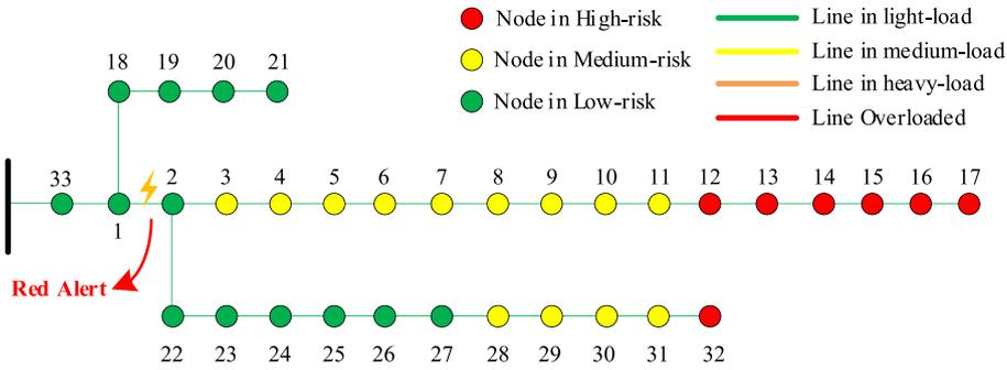
Fig. 14. The predicted risk of the nodes and lines in the distribution system in the 18th time interval.
