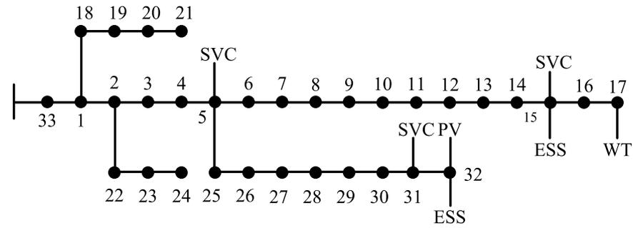
Fig. 3. The topology of IEEE 33 nodes power distribution system.
