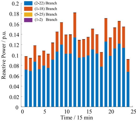
**Fig. 7.** Reactive power loss due to lightning-caused trip out.
