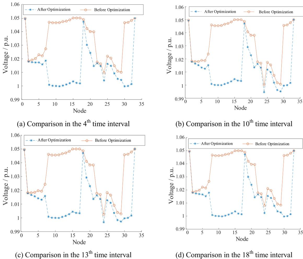
Fig. 18. Node voltage before and after optimization.
