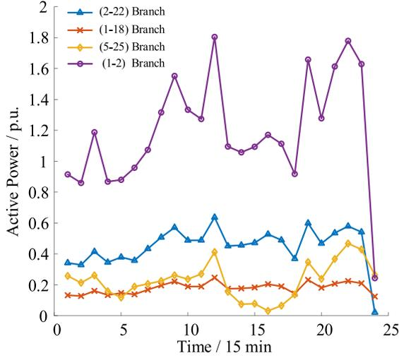
**Fig. 6.** Active power loss due to lightning-caused trip out.
