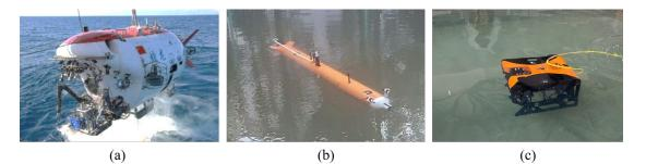
Figure 4. Underwater robot demonstration: (a) "Jiaolong" HOV [58]; (b) AUV; (c) ROV.
