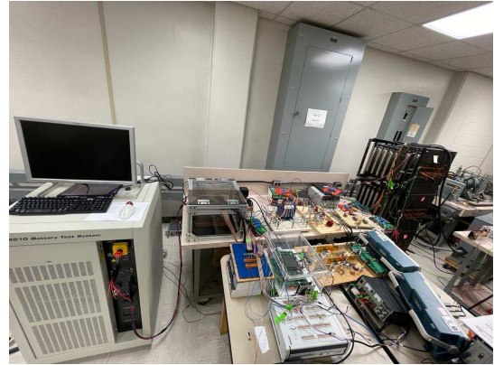
Figure 6: Three-phase grid-connected inverter with LCL filter - Hardware experimental connection.
