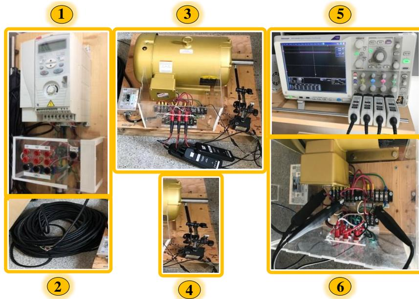
**Figure 4.8** Experimental laboratory setup of the VFD system: (1) ABB ACS150 drive with safety block, (2) power cable, (3) three-phase 7.5hp Baldor EM3710T IM with arbitrary stator windings connections and terminal voltages measurement setup, (4) bearing voltages measurement setup; (5) oscilloscope for displaying and recording output waveforms; (6) phase and CM currents measurement setup.
