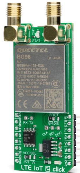
Figure 6. Picture of an "LTE IoT 2 Click" breakout board [35].
