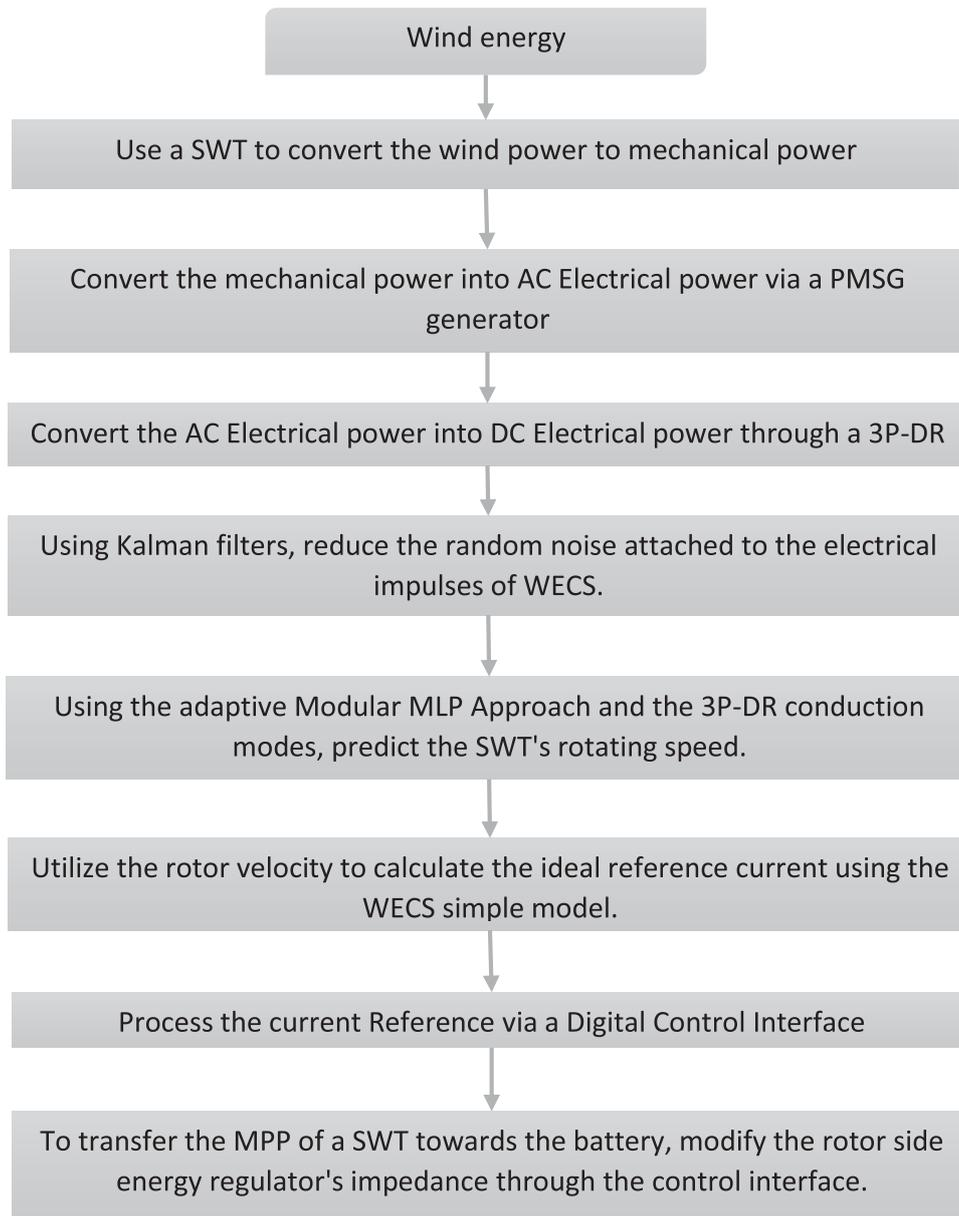
**Figure 2.** SWT uses the MPPT technique to reach its MPP.
