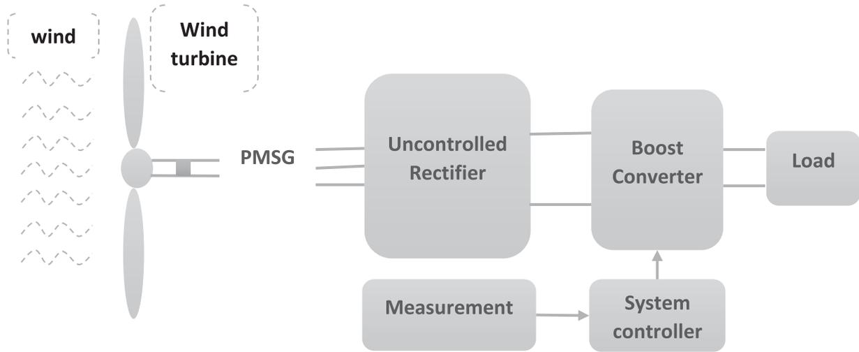
**Figure 1.** WECS configuration based on PMSG.
