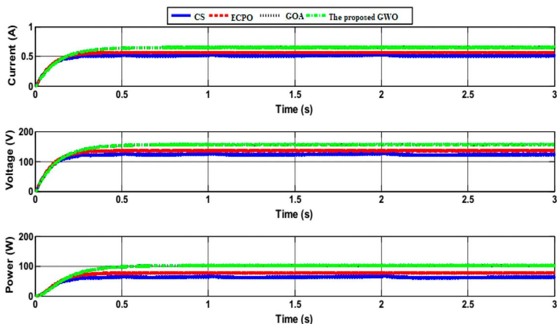
**Figure 5.** At  $V = 12$  m/s, the time responses of current, voltage and electrical power.
