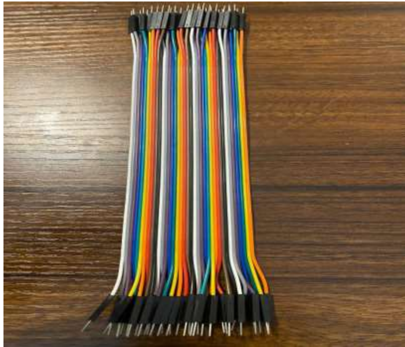
Figure 1: Shows the Jumper wires used for hardware set up connections.
