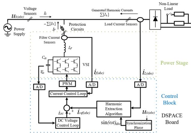
FIGURE 1. Generalized Block of Shunt APF.
