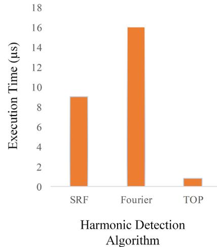
FIGURE 22. Comparison of Execution Time of Harmonic-Extraction Algorithm.
