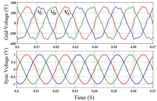
**FIGURE 8. Synchronization phase signal for TOP algorithm.**
