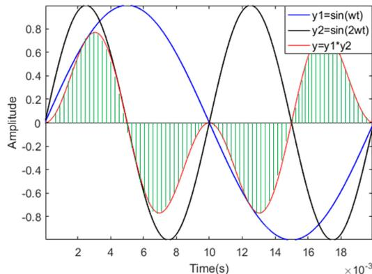
FIGURE 2. Illustration of product of trigonometric orthogonal functions.
