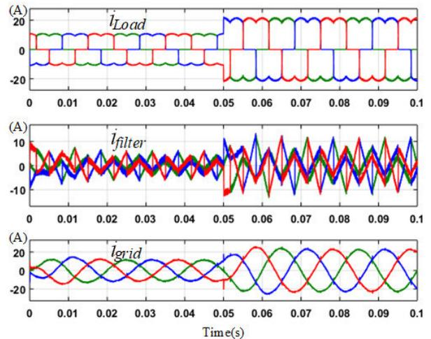
FIGURE 11. Overall compensation result of three-phase APF with TOP algorithm.
