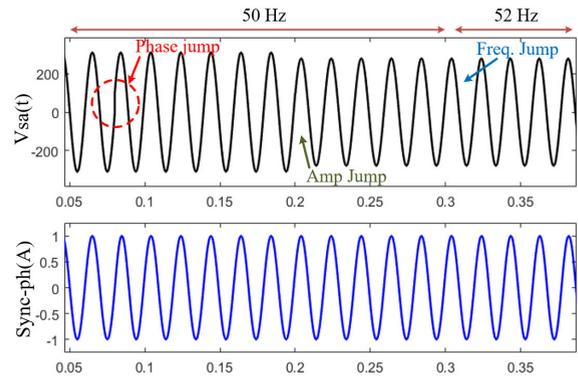
**FIGURE 9. Synchronization signal generation under different grid disturbances.**
