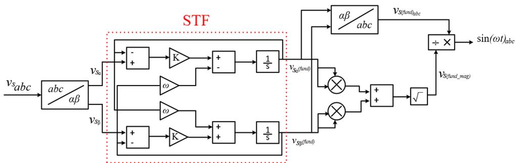
FIGURE 5. Block Diagram of synchronization phase signal.
