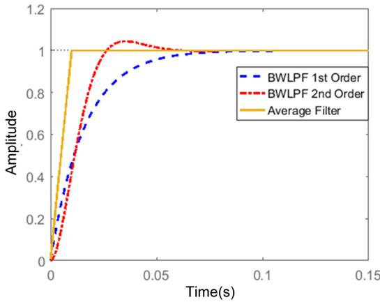
FIGURE 4. Step Response of LPF and Average Filter.
