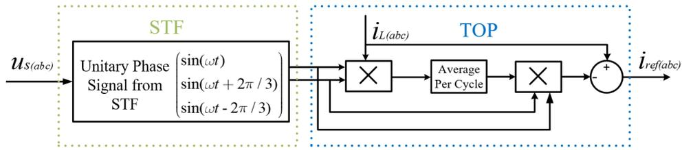
FIGURE 3. Proposed Harmonic Current Extraction Algorithm (TOP).
