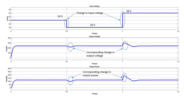
Figure 13. Simulated Line voltage regulation waveforms.
