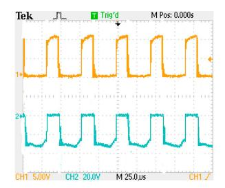
Figure 22. Diodes D<sub>1</sub>, D<sub>2</sub>, D<sub>3</sub> voltage waveform.
