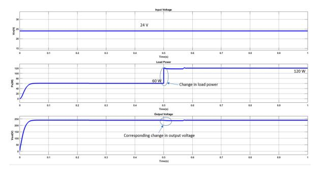
Figure 15. Simulated Load Power variation waveforms.
