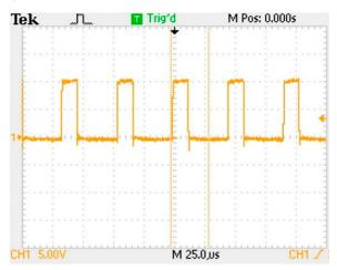
Figure 17. Gating pulse waveform.
