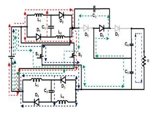
Figure 3. First mode of operation.
