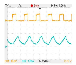
Figure 21. Inductor Current (I<sub>L1</sub>, I<sub>L2</sub>, I<sub>L3</sub>, I<sub>L4</sub>) Waveforms.
