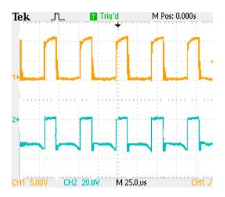
Figure 23. Diode D<sub>4</sub>, D<sub>5</sub> voltage waveform.
