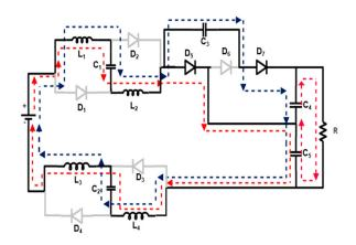
Figure 4. Second mode of operation.
