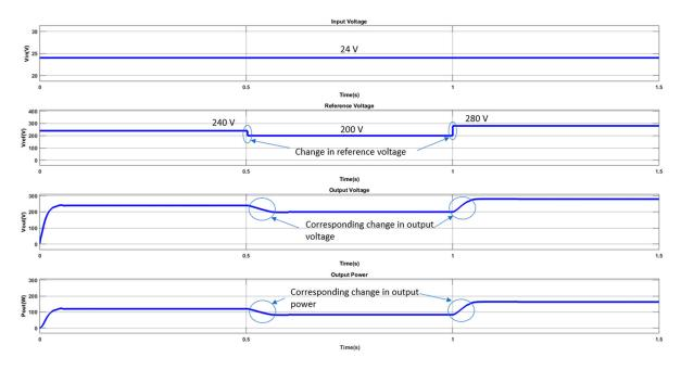
Figure 14. Simulated Reference voltage variation waveforms.
