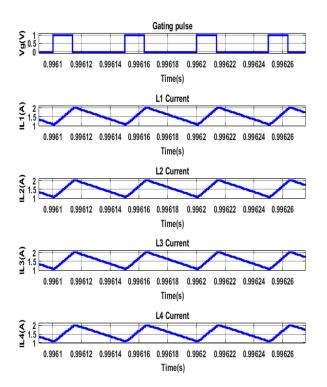
Figure 11. Simulated Inductor current waveforms.
