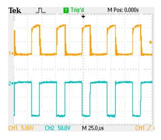
Figure 24. Diode D<sub>6</sub> voltage waveform.
