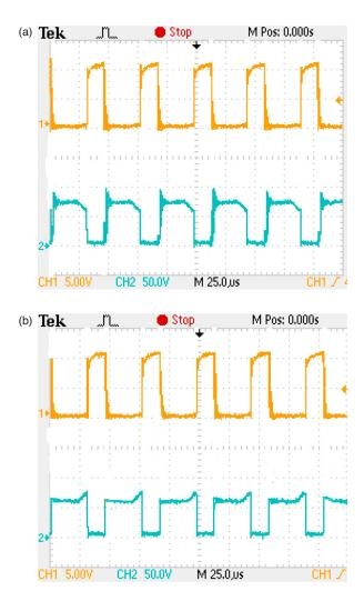
**Figure 20.** (a): Switch  $S_1$  Voltage Waveform. (b): Switch  $S_2$  voltage waveform.
