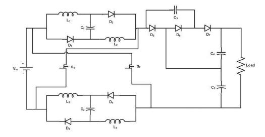
Figure 1. Proposed high-gain DC-DC converter.
