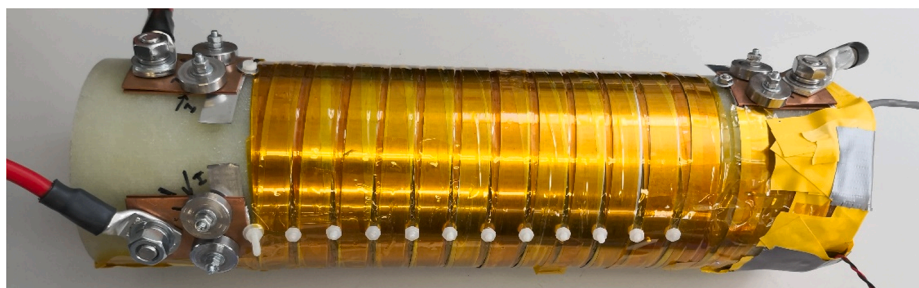
Fig. 1. Helical bifilar SFCL coil.
