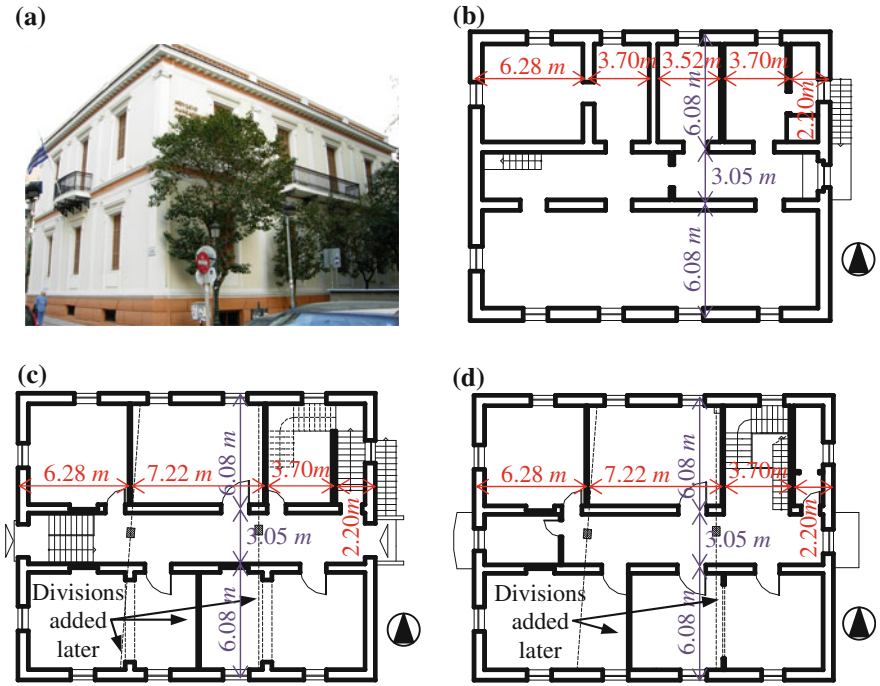
Fig. 4 The Hellenic Consulate of Thessaloniki: a South-West corner of the building, b–d plan views of the building’s basement, 1st and 2nd storey, respectively. Built in 1898 according with the designs of Ernst Ziller; sponsored by A. Syggros to house the Hellenic Consulate of Thessaloniki while the city was still under Ottoman rule. After the annexation of Thessaloniki to Greece, the building operated as a primary school [11, 12]
