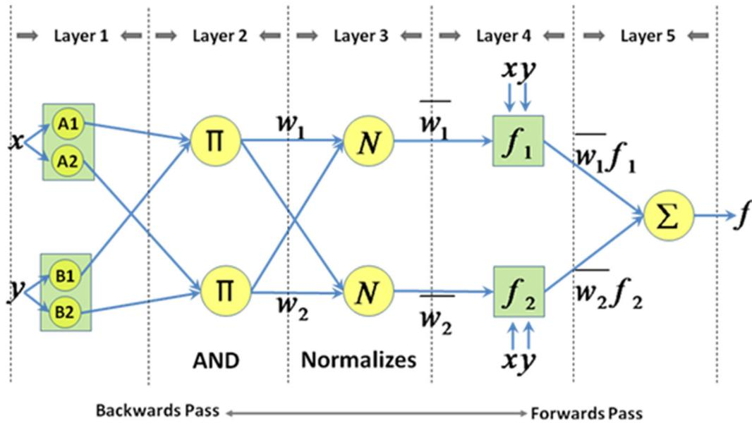
Fig. 3. (a) A two-input first-order Sugeno fuzzy model with two rules; (b) An equivalent ANFIS structure.
