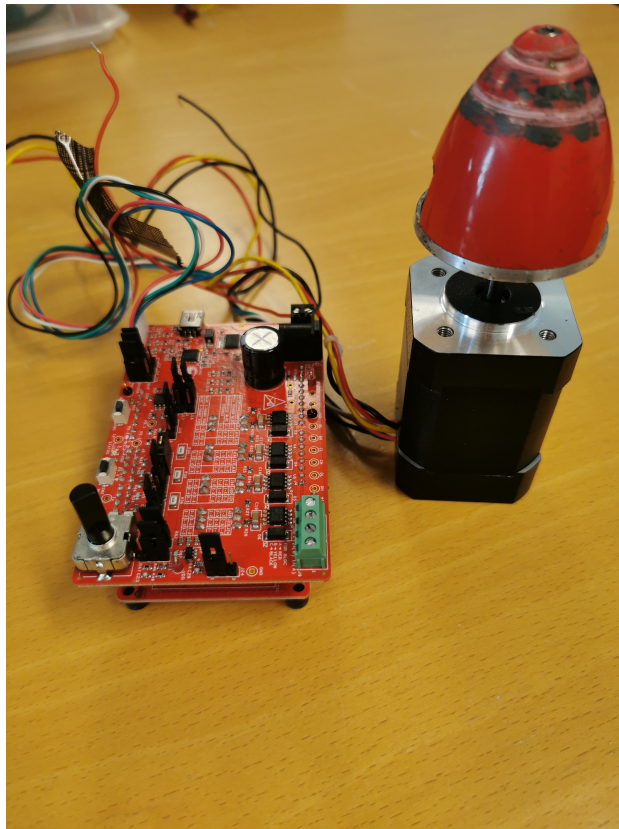
Figure 6: The Cypress motor kit. To the left is the motor control evaluation board and to the right is the BLY172S-24V-4000 BLDC motor.
