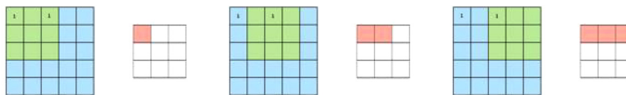
Fig. 1. An example of Sparse convolution. Given the sparsity of the matrix, convolution operations are performed exclusively around the non-zero elements (3 in total).
