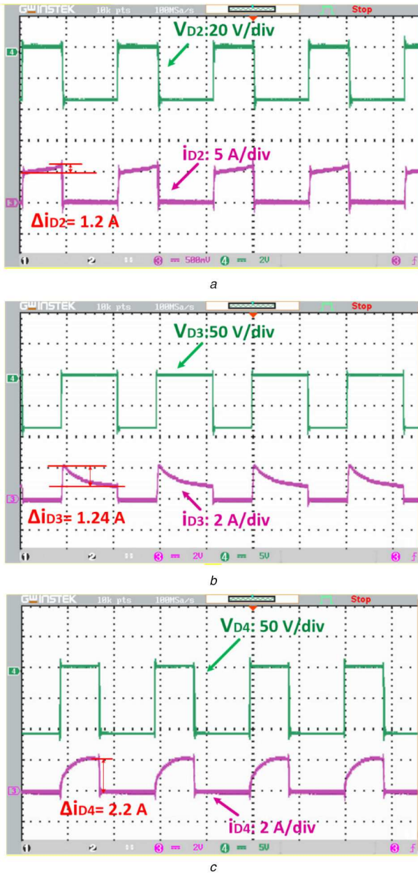
Fig. 13 Experimental results of the SSQBCI, (Time/Dive = 10 us/div) (a) V_{D2} and i_{D2} , (b) V_{D3} and i_{D3} , (c) V_{D4} and i_{D4} , (d) V_{D5} and i_{D5}
