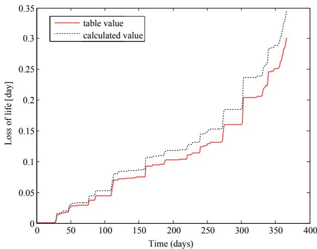
Fig. 7. LOL by IEC model with standard and calculated time constants.
