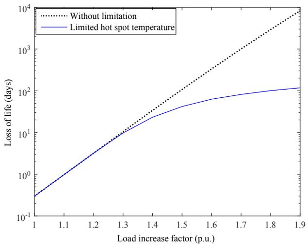
Fig. 11. Loss of life calculation for increased load with and without limited hotspot temperature.
