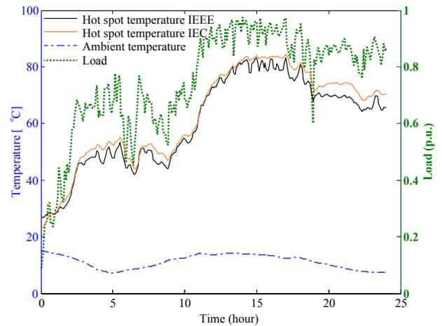
Fig. 3. Hot spot temperature calculated using IEEE and IEC models 2016-06-08.
