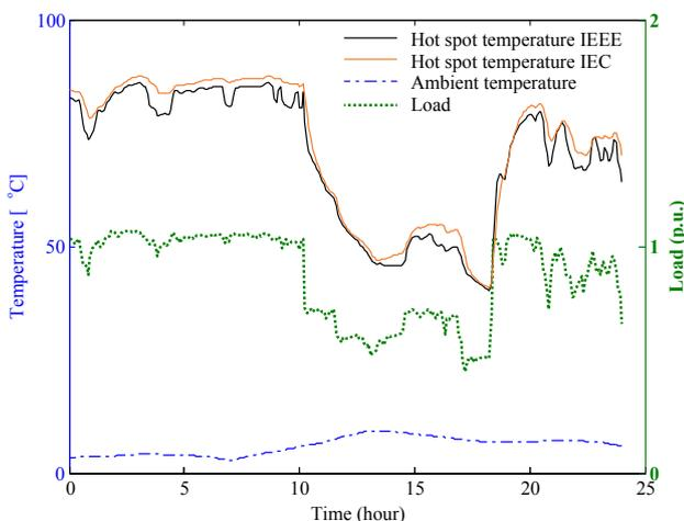
Fig. 2. Hot spot temperature calculated using IEEE and IEC models 2016-10-29.
