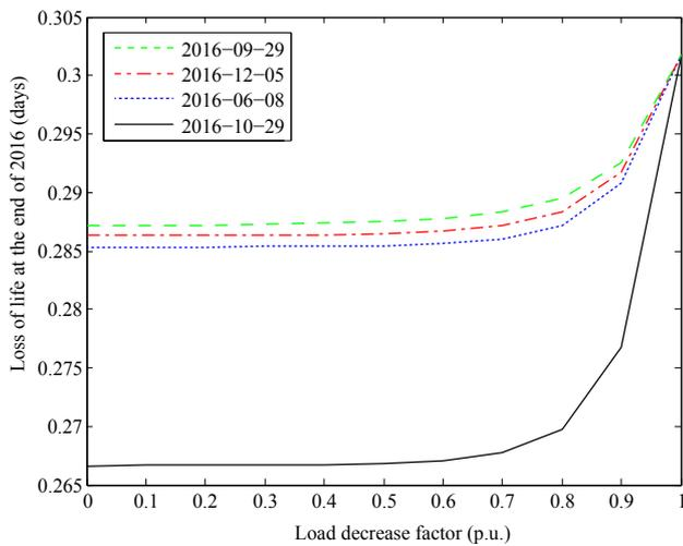
**Fig. 8.** Loss of life calculation in IEC model for decreased load at critical days.
