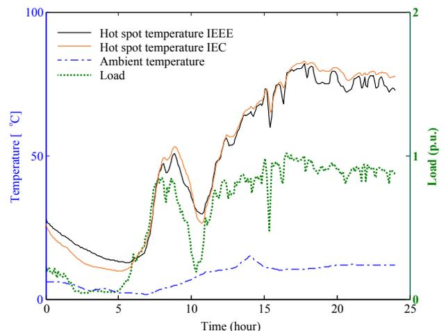
Fig. 5. Hot spot temperature calculated using IEEE and IEC models 2016-09-29.
