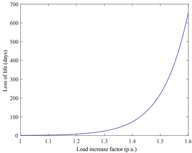
Fig. 10. Loss of life for different increasing factor by considering 8 °C safety margin.
