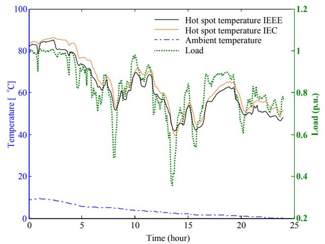
Fig. 4. Hot spot temperature calculated using IEEE and IEC models 2016-12-05.
