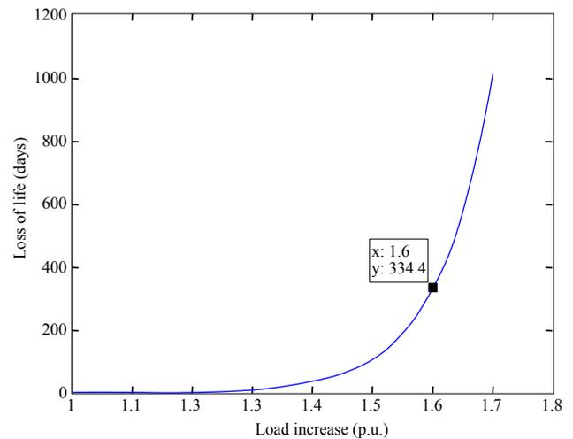
**Fig. 9.** Loss of life calculation in IEC model for increasing load.
