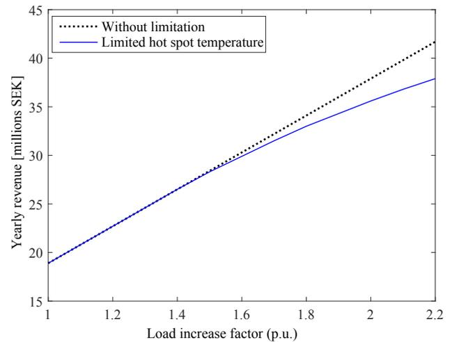
Fig. 12. Revenue comparison for increased load with and without limited hot spot temperature.
