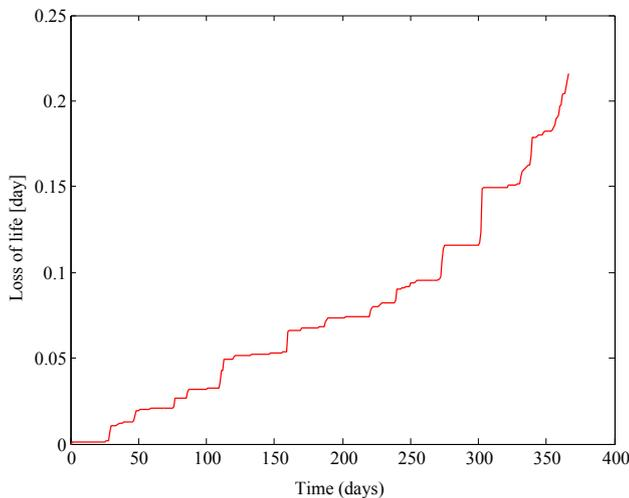
Fig. 6. Daily loss of life calculated by IEEE thermal model.
