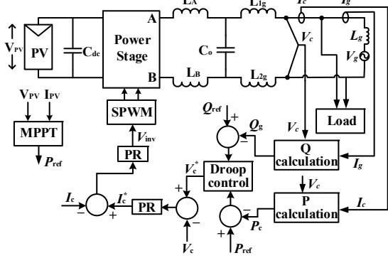
Fig 4. Droop based multifunctional control strategy for transformerless PV system.
