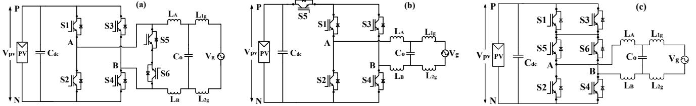
Fig 3. Existing Single-phase transformerless topologies for PV application: (a) HERIC topology (b) H5 topology (c) H6 type topology.
