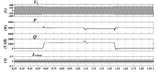
Fig 11. Power flow and leakage current when 0.09pu grid voltage sag remain more than  $t_c$ .
