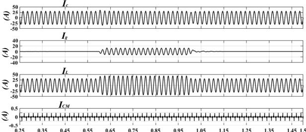
Fig 9. Performance of the transformerless system when the local load suddenly increases than MPPT.
