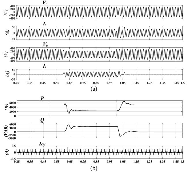
Fig 12. Performance of the transformerless PV system with 0.3pu grid voltage sag: (a) output characteristics (b) power flow and leakage current.
