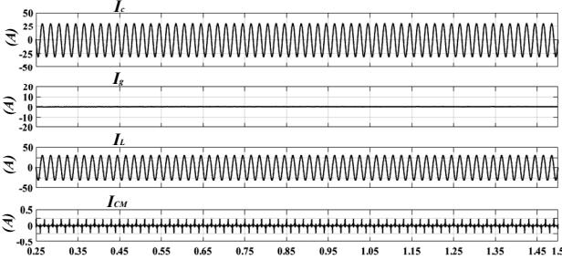
Fig 8. Steady state operation when the local load meets the MPPT.
