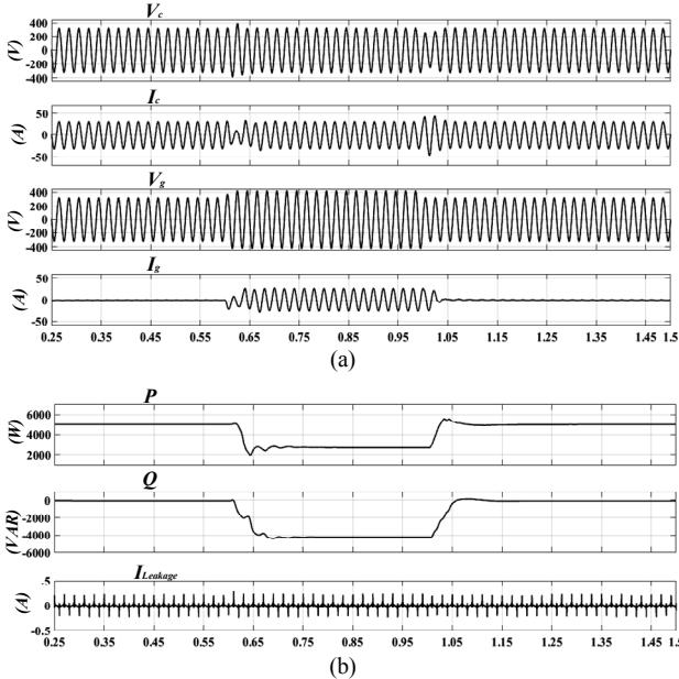
Fig 13. Performance of the transformerless PV system with 0.3pu grid voltage swell: (a) output characteristics (b) power flow and leakage current.
