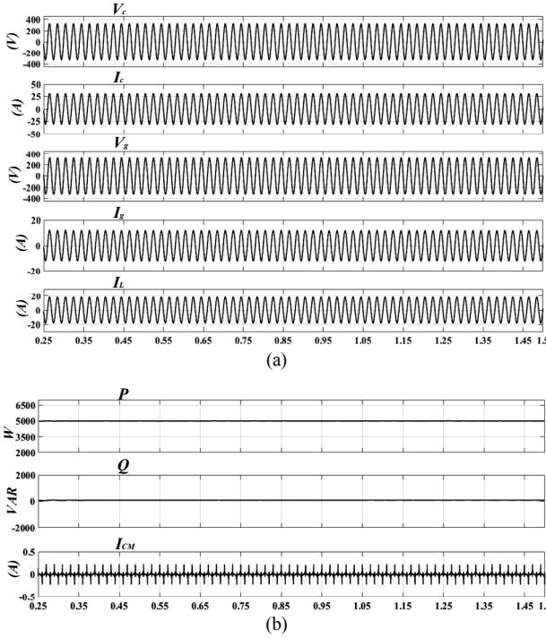
Fig 7. Steady state operation: (a) output voltage  $V_c$ , output current  $I_c$ , grid voltage  $V_g$ , grid current  $I_g$ , and load current  $I_L$  (b) real power  $P$ , reactive power  $Q$ , and leakage current  $I_{CM}$ .
