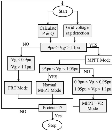
Fig 6. Control flowchart of the droop based multifunctional control strategy for transformerless PV application.
