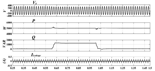
Fig 10. Power flow and leakage current with 0.09pu grid voltage sag.
