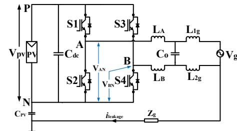
Fig 2. Single-phase transformerless FB inverter for grid-tied PV system.
