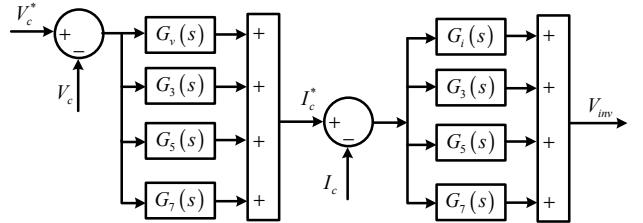
Fig 5. Block diagram of the PR+HC controller.
