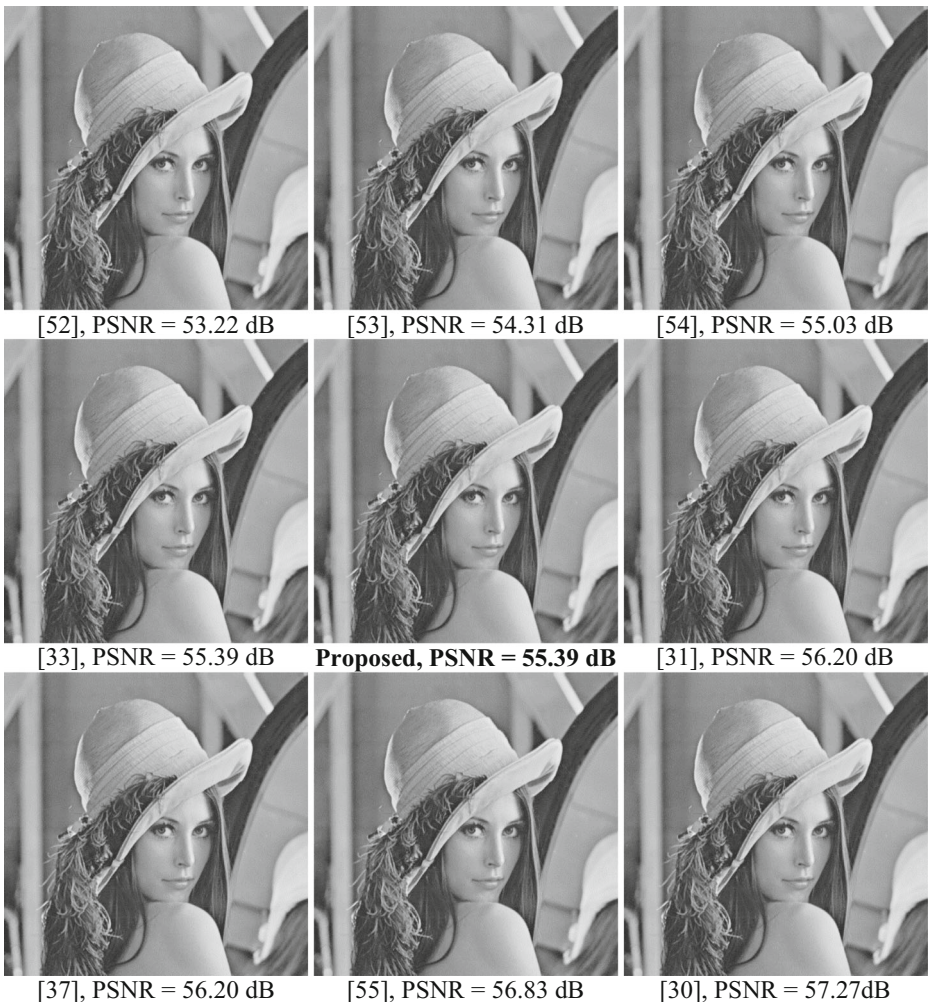
Fig. 5 Performance comparison of the proposed data hiding algorithm with other proposed algorithms in Lena with the embedding data of 20 Kbits
