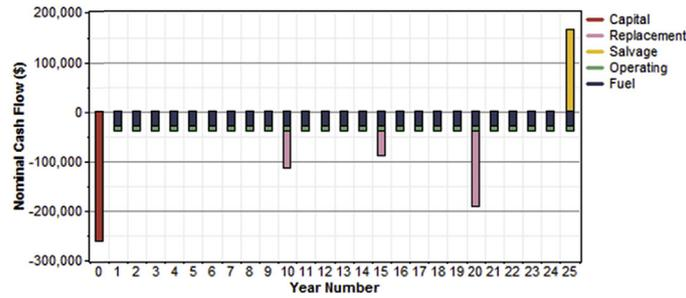
(c) Diesel-Solar PV-BESS mix
