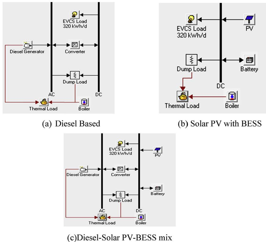
**Fig. 7.** Optimal EVCS configurations in Case-1: Isolated EVCS.
