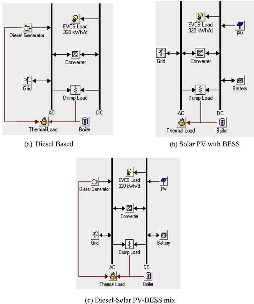
Fig. 8. Optimal EVCS configurations in Case-2: Grid connected EVCS.
