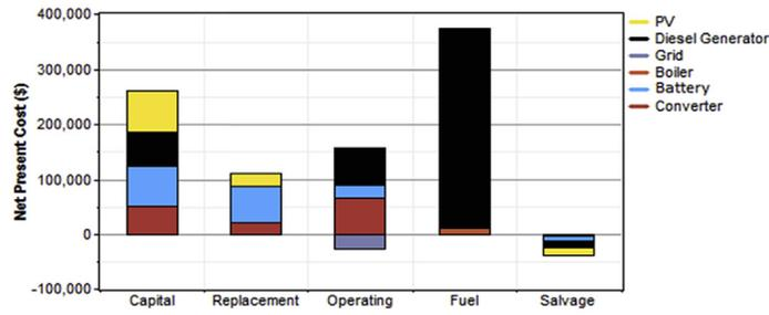
(c) Diesel-Solar PV-BESS mix
