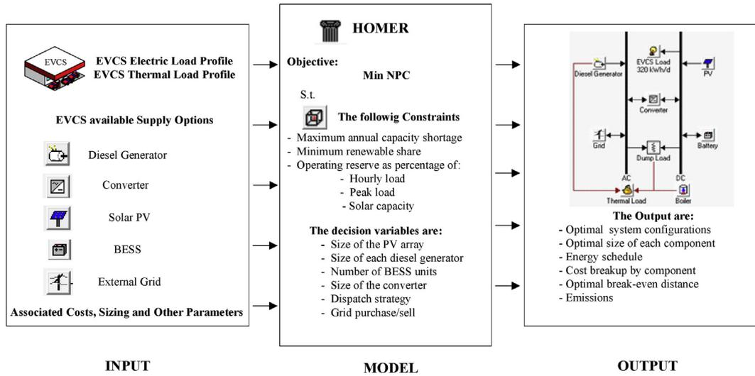
Fig. 1. Architecture of EVCS design using HOMER [12].
