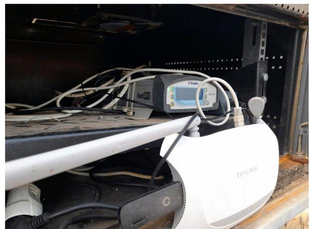
Figure 3. Trimble NetR9 GNSS reference receiver with remote connections.
