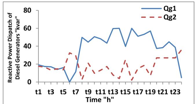
Fig. 8. Reactive power dispatch of diesel generators (Case 2).
