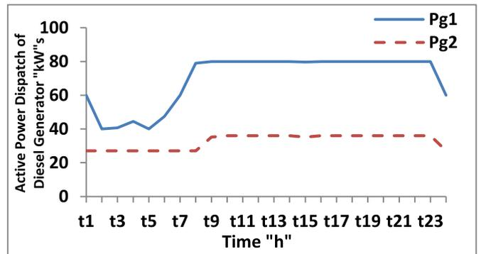
Fig. 7. Active power dispatch of diesel generators (Case 1).
