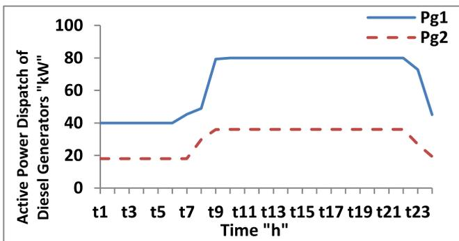
Fig. 15. Active power dispatch of diesel generators (Case 4).
