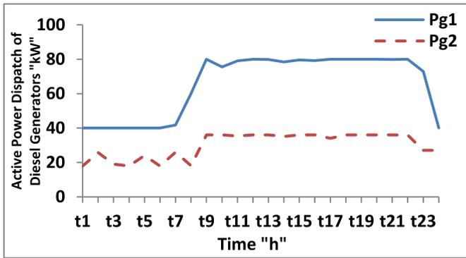
Fig. 9. Active power dispatch of diesel generators (Case 2).
