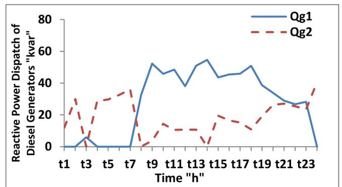
Fig. 13. Reactive power dispatch of diesel generators (Case 4).
