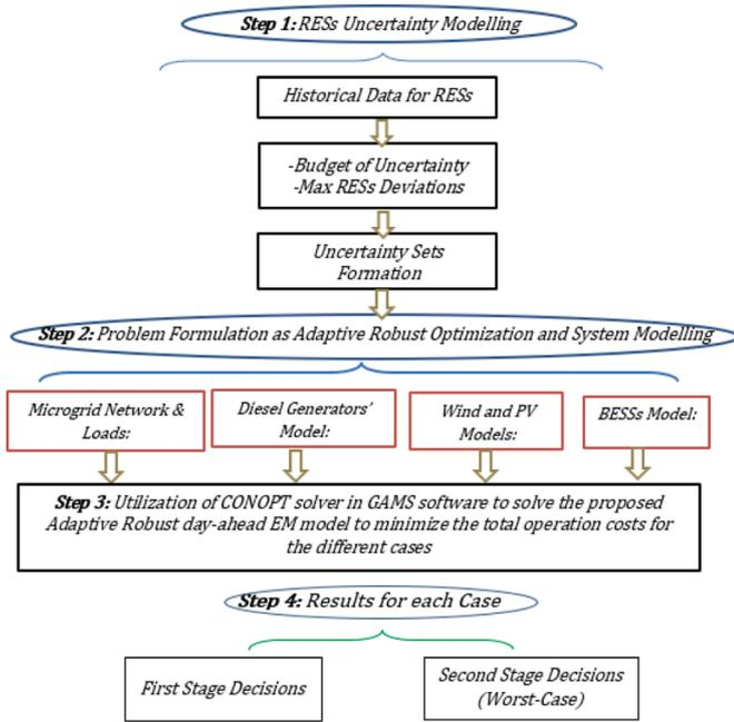
Fig. 5. Framework of the proposed adaptive robust energy management model and solution procedure.
