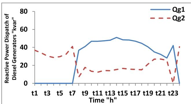
Fig. 11. Reactive power dispatch of diesel generators (Case 3).
