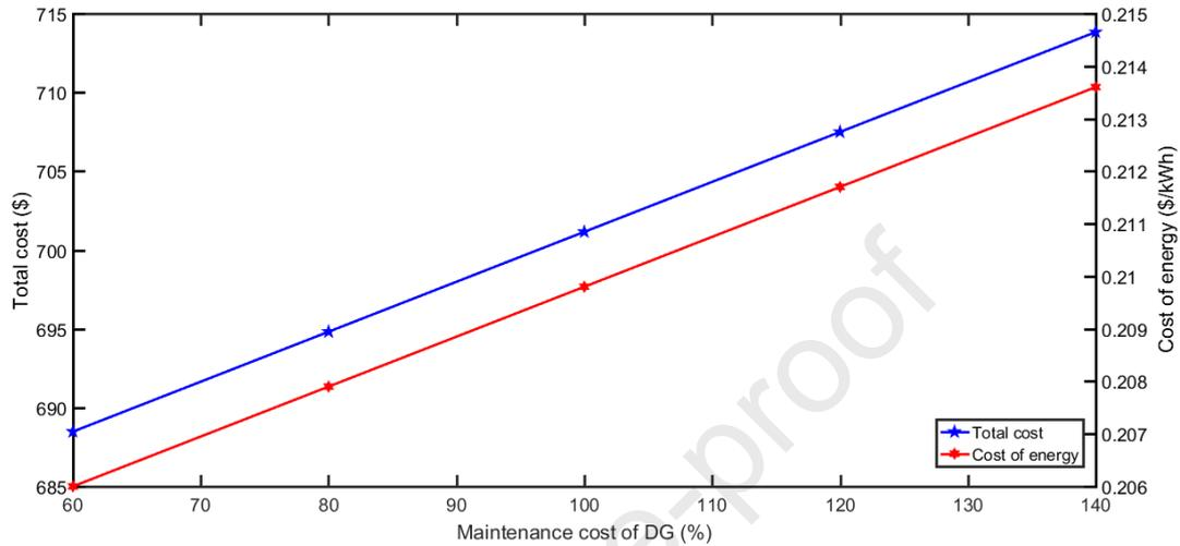
Fig. 27a. Effect of maintenance cost of DG on TC and COE
