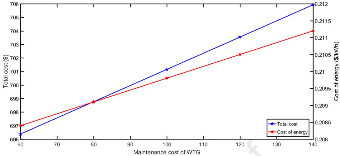
Fig. 27c. Effect of maintenance cost of WTG on TC and COE
