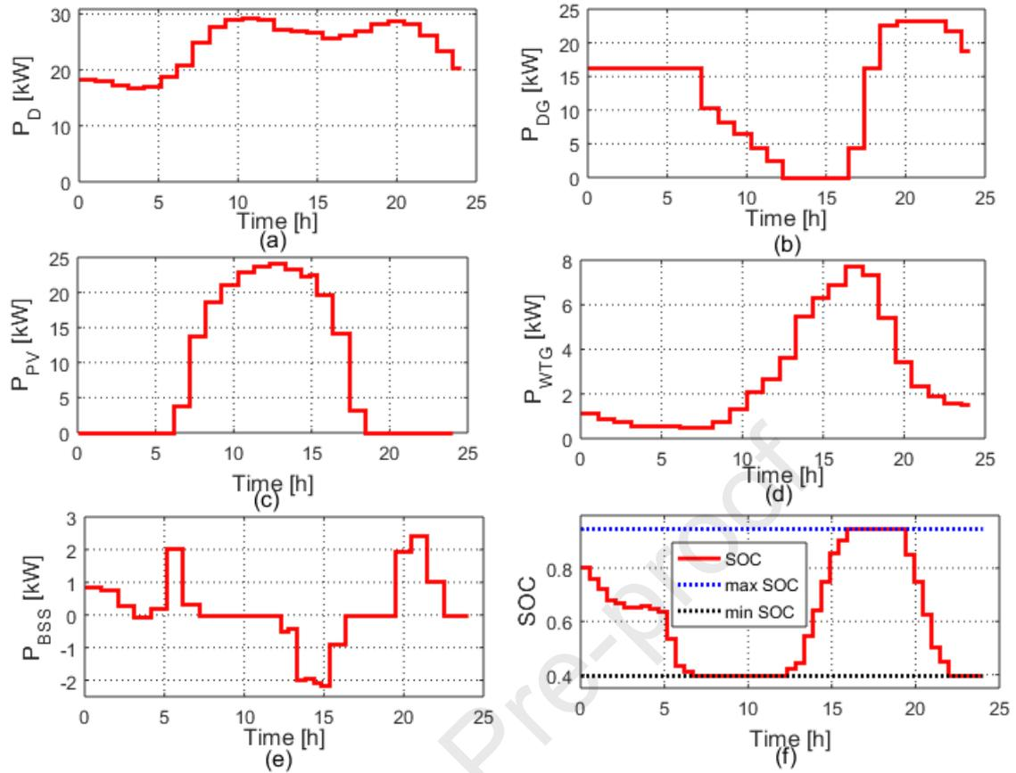
Fig. 13. Autumn weekday power flow and load profile: (a) Power demand, (b) DG power output, (c) PV power output, (d) WTG power output, (e) BSS power output and (f) SOC.
