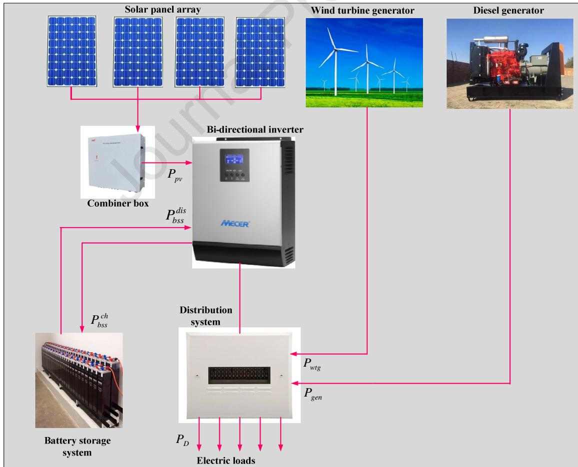
Fig. 2. Configuration of the PV-WTG-BSS-DG MGS
