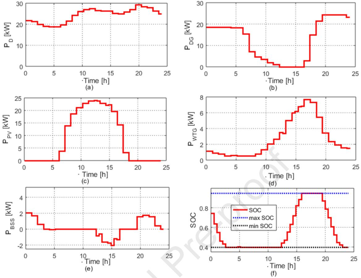
Fig. 16. Autumn weekend power flow and load profile: (a) Power demand, (b) DG power output, (c) PV power output, (d) WTG power output, (e) BSS power output and (f) SOC.
