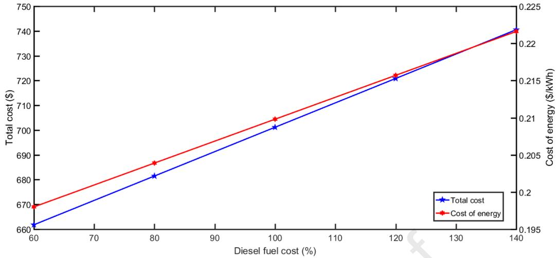
Fig. 25. Effect of diesel fuel cost on TC and COE
