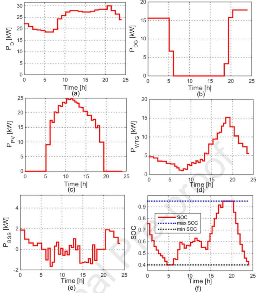
Fig. 12. Summer weekend power flow and load profile: (a) Power demand, (b) DG power output, (c) PV power output, (d) WTG power output, (e) BSS power output and (f) SOC.
