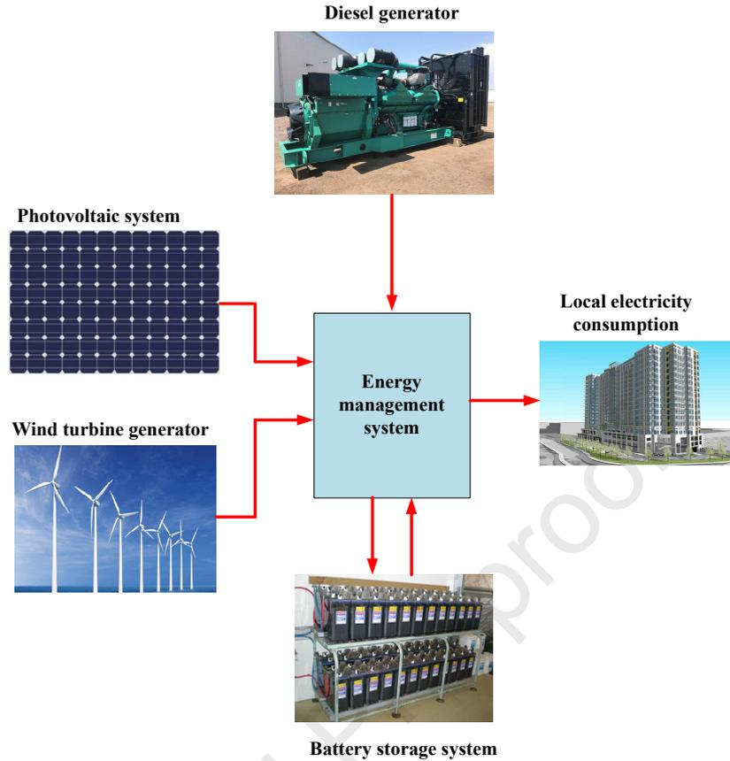
Fig. 1. Proposed electricity generation configuration for small autonomous networks.
