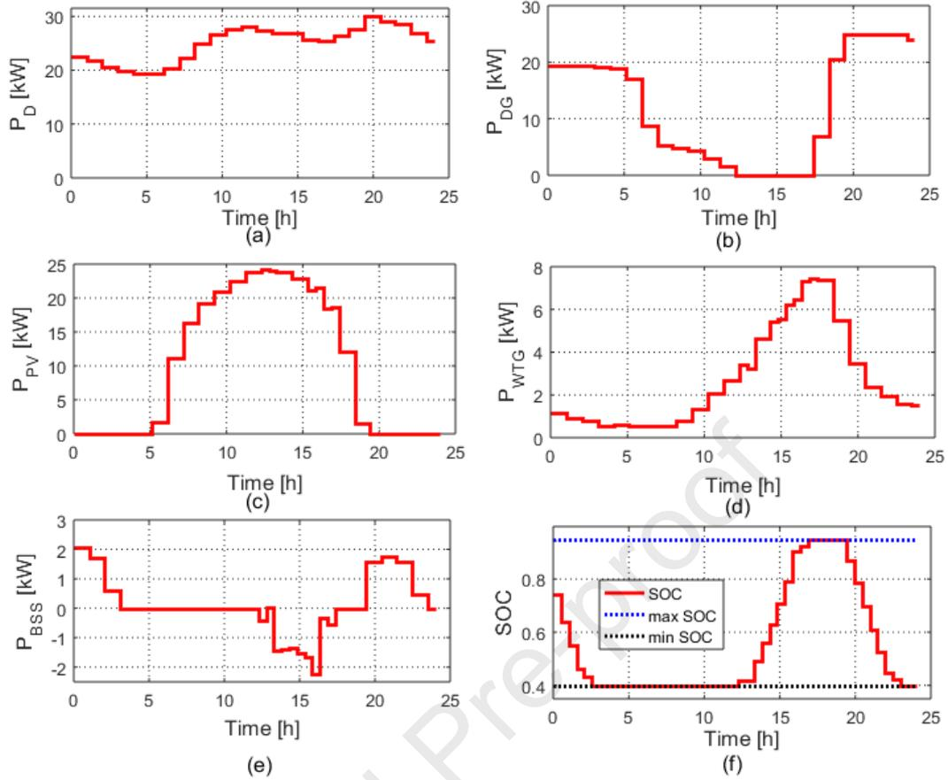
Fig. 24. Spring weekend power flow and load profile: (a) Power demand, (b) DG power output, (c) PV power output, (d) WTG power output, (e) BSS power output and (f) SOC.
