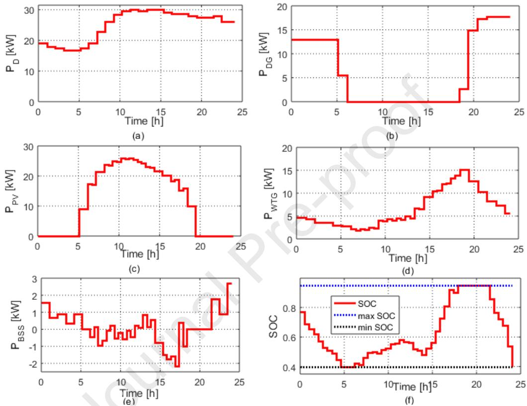
Fig. 5. Summer weekday power flow and load profile: (a) Power demand, (b) DG power output, (c) PV power output, (d) WTG power output, (e) BSS power output and (f) SOC.
