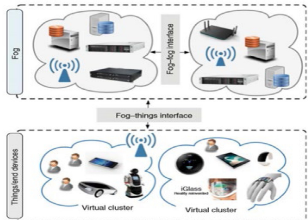
Fig. 2. Architecture of two-tier model of fog [4].
