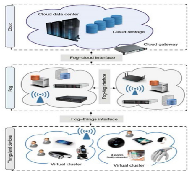
Fig. 1. Architecture of three-tier model of fog [4].
