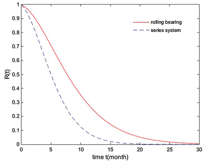
Fig. 3. Reliability of the system given that both rolling bearings enter state 1 at time 0.
