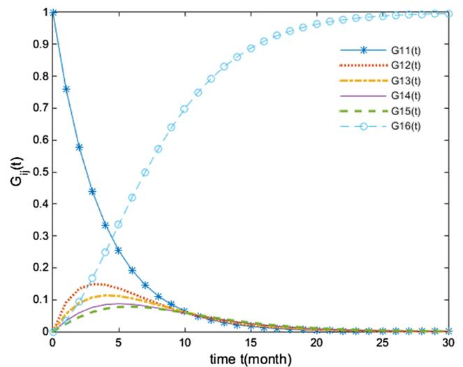
Fig. 4. Probabilities of transferring to state 1, 2, 3, 4, 5, 6 at time  $t$  when the rolling bearing is in state 1 at  $t = 0$ .
