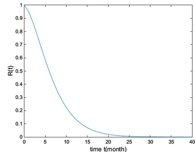
Fig. 2. Reliability of the rolling bearing given that the rolling bearing enters state 1 at time 0.
