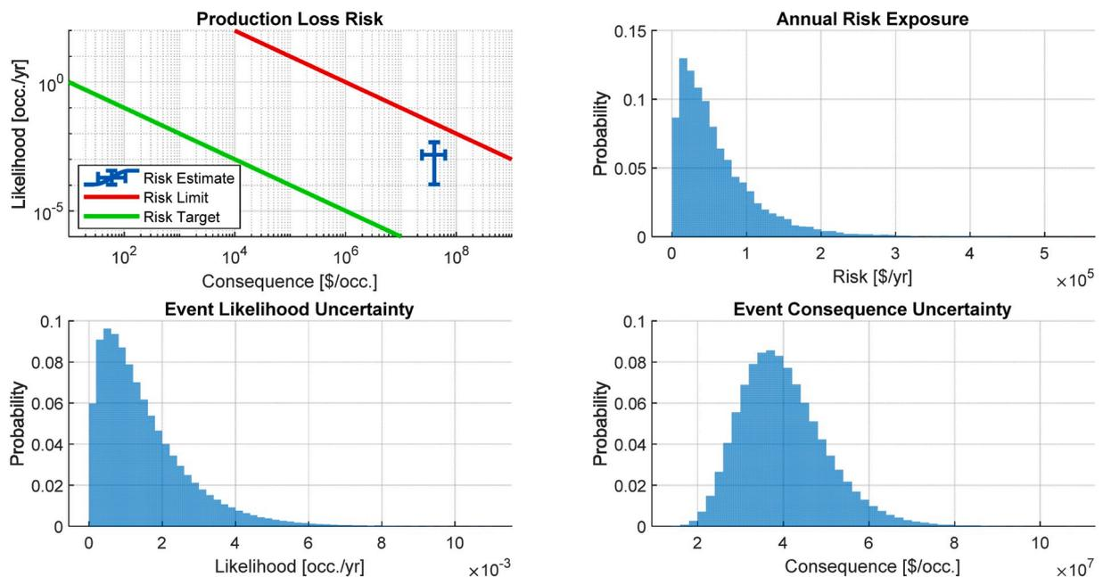
Fig. 13. Gas leak - loss of production - baseline risk results.
