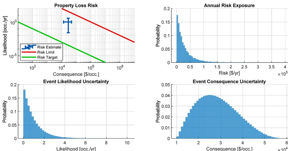
Fig. 16. Compressor failure - loss of property - baseline risk results.
