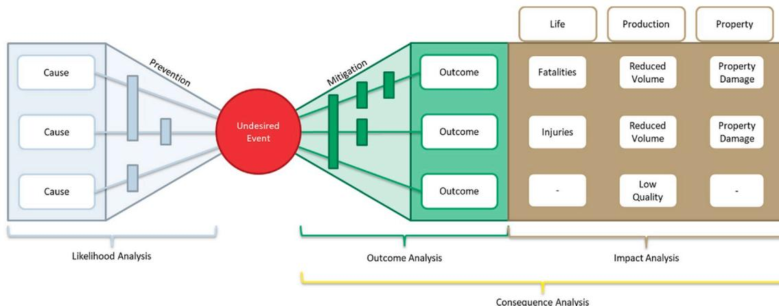
Fig. 4. Bowtie analysis schematic.
