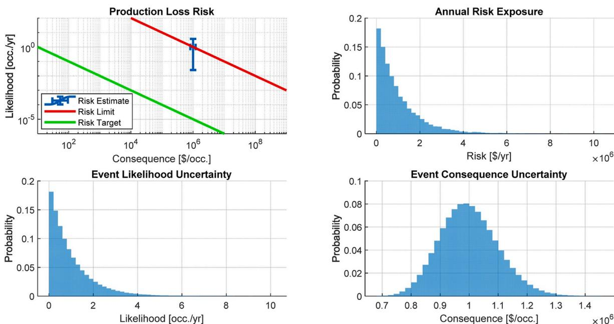
Fig. 15. Compressor failure - loss of production - baseline risk results.
