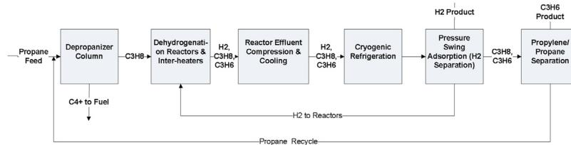
**Fig. 3 – Block diagram of UOP OLEFLEX propane dehydrogenation (PDH) process.**
