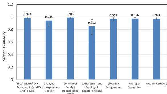
**Fig. 6 – Section availability of individual process blocks for a proposed PDH process.**
