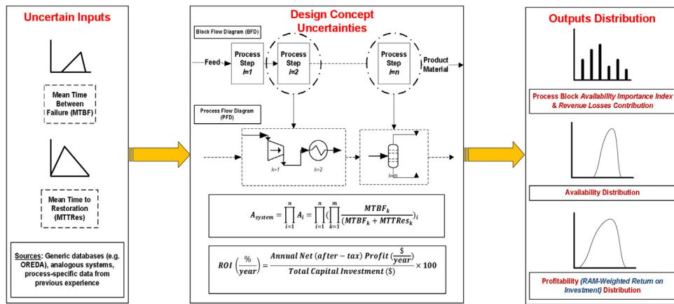
Fig. 2 – Uncertainty propagation of process RAM characteristics.
