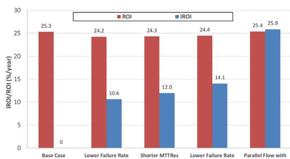
**Fig. 9 – Comparison of ROI and IROI for alternative design scenarios of a PDH process compression system.**
