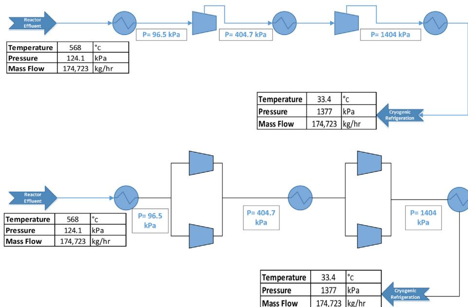
**Fig. 8 – Compression and cooling section configurations for (top) base case design and modifications 1-3, and (bottom) modification 4 (parallel flow arrangement).**
