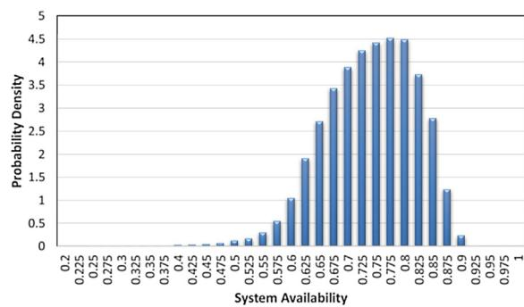
**Fig. 4 – Probability density graph of overall PDH process availability.**
