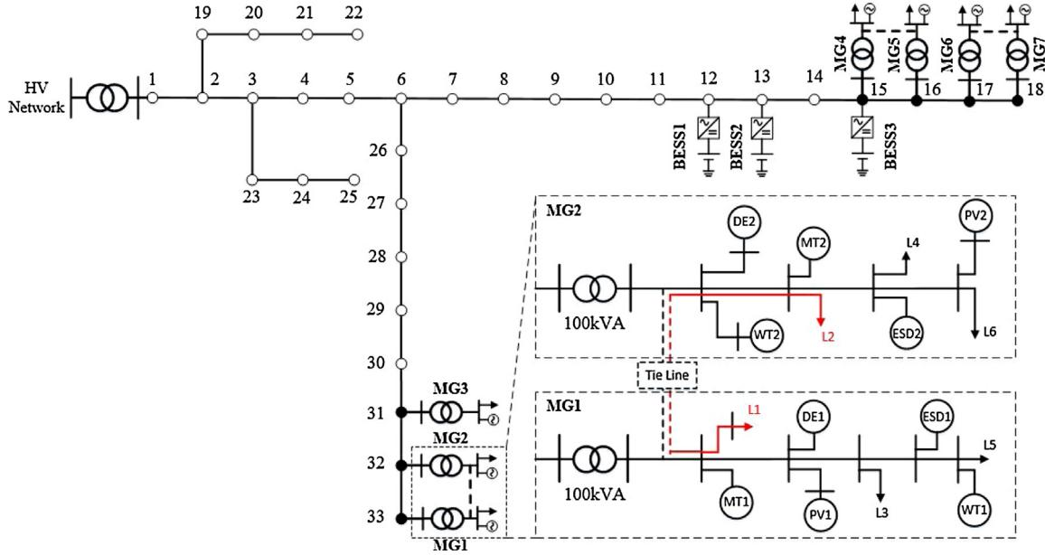
Fig. 4. 33-bus test distribution system with CHP-based MMGs.
