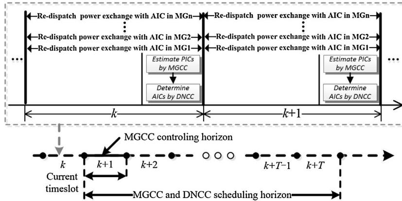
Fig. 2. Timeline for the sequential coordination of MGCC and DNCC in a DN, including coupled microgrids.
