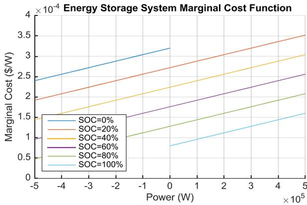
Fig. 4. Energy storage system marginal cost function.
