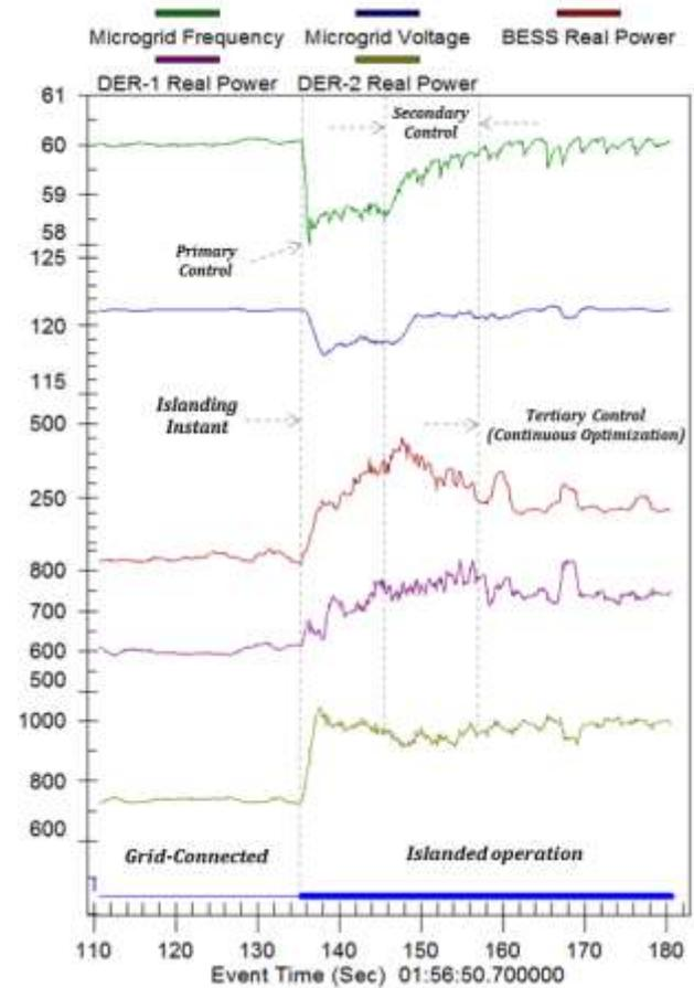
Fig. 18. Experimental islanding – distributed optimization performance.
