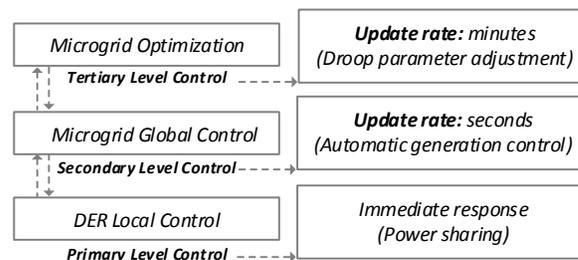
Fig. 1. Hierarchical control of a microgrid.
