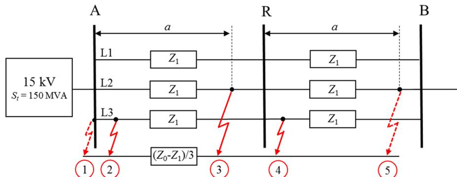
**Fig. 8.** Equivalent diagram of various cases of tested double phase-to-earth faults.
