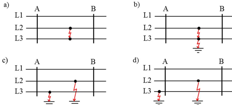
Fig. 4. Examples of various two phase or double phase-to-earth faults in MV power lines.
