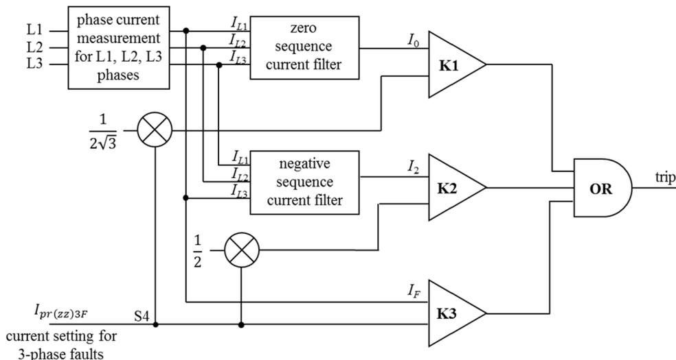
Fig. 6. Operation principle of the overcurrent protection against multi-phase faults including negative and zero sequence current criteria.
