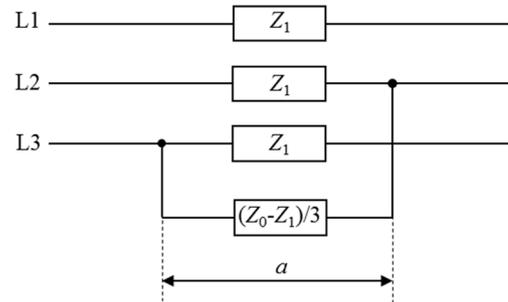
Fig. 5. Part of the fault current circuit loop related to a cross-country fault occurring between phases L2 and L3 within the  $a$  distance.
