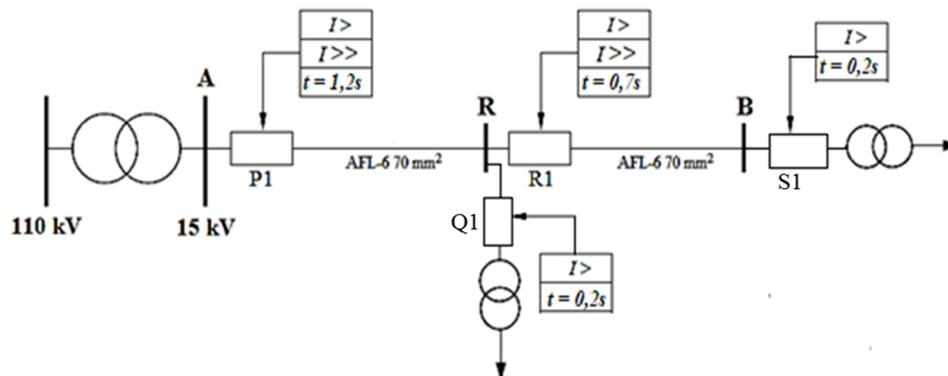
Fig. 7. Diagram of the 15 kV test system adopted for simulations.
