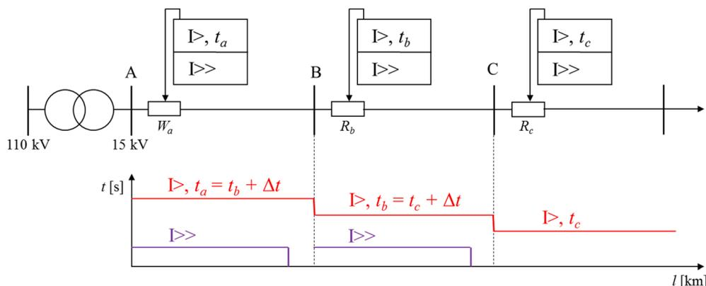
Fig. 1. Coordination example of  $I >$  time-delay overcurrent protection relays' settings with appropriate current settings of  $I \gg$  short-circuit protection in MV lines.
