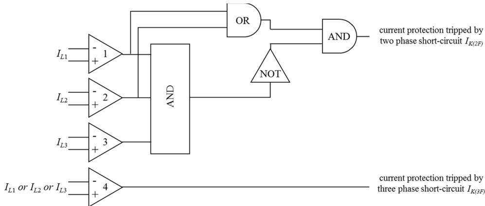
Fig. 3. Diagram for short-circuit type differentiation. Comparators 1, 2 and 3 are set for two phase short-circuits ( $F2nast$ ) and comparator 4 is set for three phase short-circuits ( $F3nast$ ).
