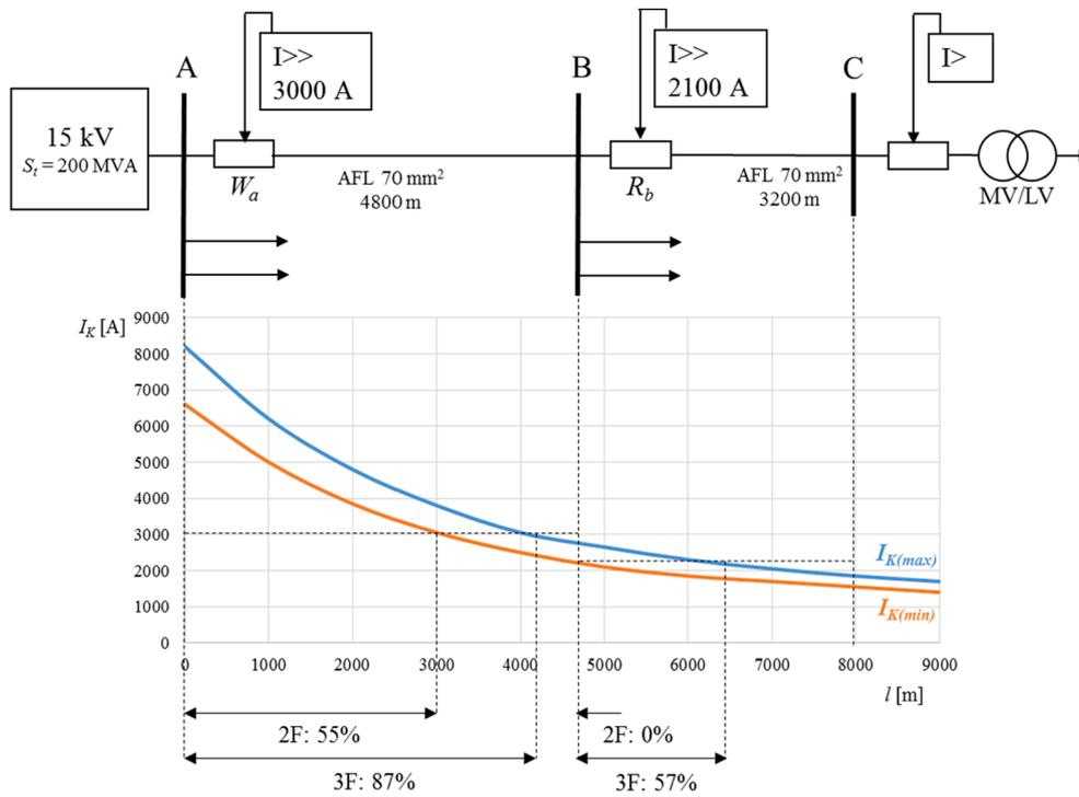
Fig. 2.  $I_{\gg}$  protection operation zones installed in A and B substations during three phase ( $I_{K(max)}$ ) and two phase ( $I_{K(min)}$ ) short-circuits in a 15 kV line supplied from a substation with a short-circuit power  $S_t = 200$  MVA.
