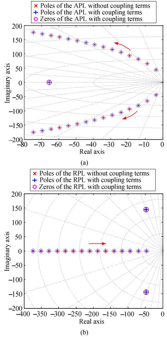
Fig. 4. Root locus plot of the APL and RPL with and without coupling terms. (a) The APL with  $K_{ip}$  varies from 0.005 to 0.1. (b) The RPL with  $K_{iq}$  varies from 0.045 to 0.03.
