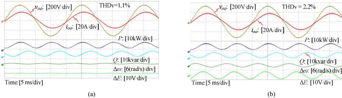
Fig. 14. Experimental results when VSG works in the standalone mode with 100% unbalanced resistive-inductive loads ( $18+j3 \Omega$  load in phase A, no load in phase B and phase C). (a)  $f_{pc} = 22$  Hz,  $f_{gc} = 8.6$  Hz (b)  $f_{pc} = 35$  Hz,  $f_{gc} = 20$  Hz.
