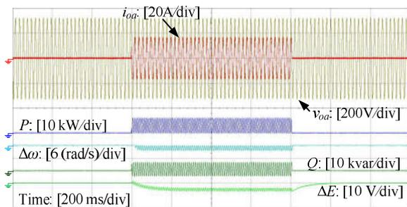
Fig. 15. Dynamic waveform of the VSG operating in the standalone mode with load in phase A steps between no load and  $18+j3 \Omega$ .
