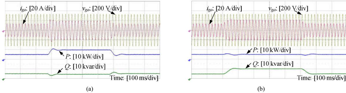
Fig. 10. Dynamic responses with  $K_{ip} = 0.06$ ,  $K_{iq} = 0.045$  when (a) Grid frequency drops 1% and then returns back to its nominal value. (b) The amplitude of grid voltage drops 5% and then returns back to its nominal value.
