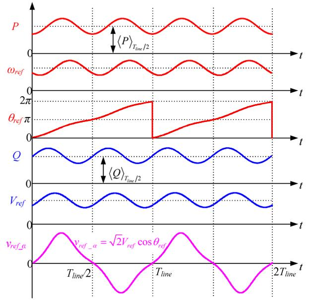
Fig. 2. DLFR in the instantaneous output power distort the PWM reference of the VSG
