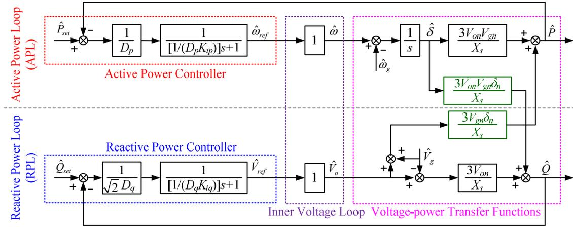
Fig. 3. Line-frequency-averaged small-signal model of the VSG
