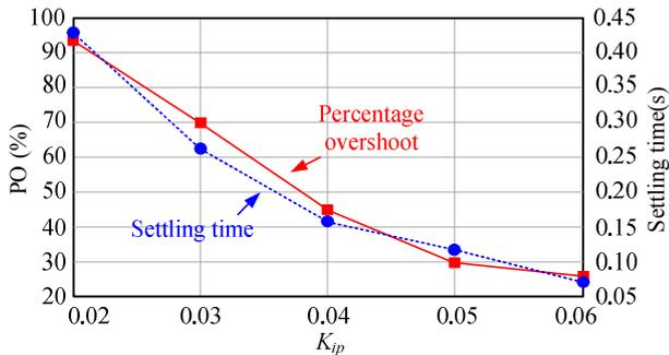
Fig. 11. Settling time and percentage overshoot of the active power when grid frequency drops 1% with  $K_{ip}$  varies.
