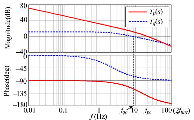
Fig. 7. Bode diagram of the loop gain.
