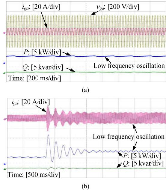
Fig. 12. Experimental results with  $K_{ip} = 0.005$ ,  $K_{iq} = 0.045$ . (a) Steady-state with  $P_{set} = 3$  kW,  $Q_{set} = 0$  var. (b) Dynamic waveform when grid frequency drops 0.6%.
