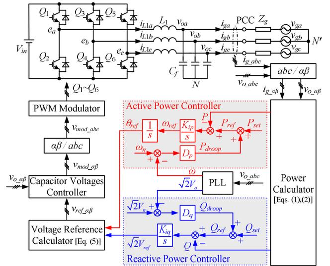
Fig. 1. Topology and control diagram of the VSG.
