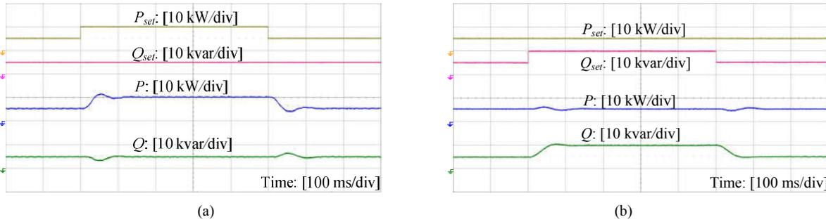
Fig. 9. Dynamic responses with  $K_{ip} = 0.06$ ,  $K_{iq} = 0.045$  when (a)  $P_{set}$  steps between 5 kW and 10 kW. (b)  $Q_{set}$  steps between 5 kvar and 10 kvar.
