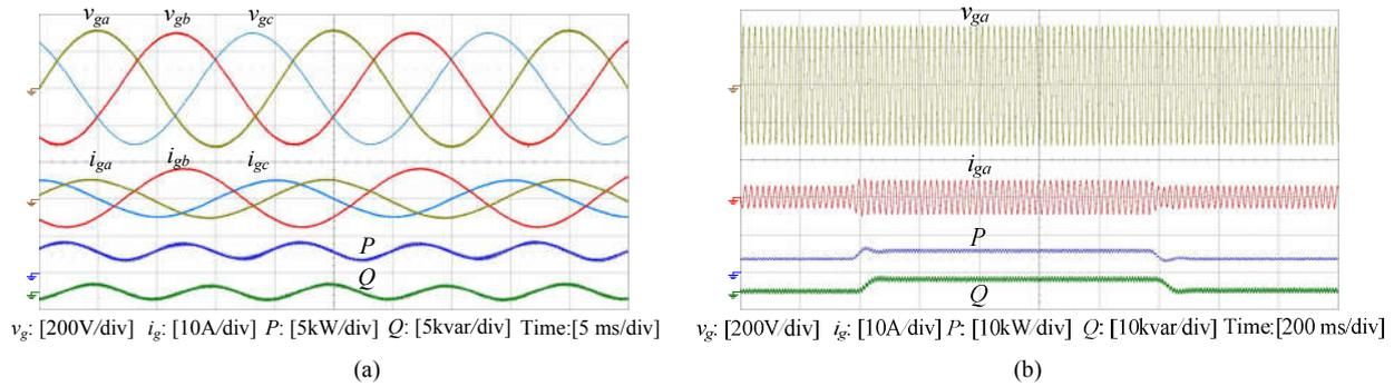
Fig. 13. Steady-state and dynamic waveforms of the VSG under unbalanced grid voltage condition. (a) Steady-state with  $P_{set} = 3$  kW,  $Q_{set} = 0$  var. (b) Dynamic waveform with power demands step between  $P_{set} = 3$  kW,  $Q_{set} = 0$  var and  $P_{set} = 6$  kW,  $Q_{set} = 3$  kvar.
