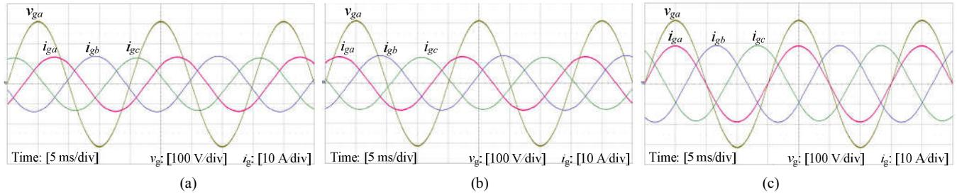
Fig. 8. Steady-state experimental results with  $K_{ip} = 0.06$ ,  $K_{iq} = 0.045$ . (a)  $P_{set} = 5$  kW,  $Q_{set} = 5$  kvar (inductive). (b)  $P_{set} = 5$  kW,  $Q_{set} = -5$  kvar (capacitive). (c)  $P_{set} = 10$  kW,  $Q_{set} = 0$  var.
