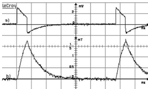
**Fig. 3** **a** Waveform of the electrical field induced in the pick-up coil probe described in the text, **b** waveform of the induced magnetic field
