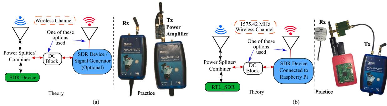
Fig. 12. Pluto SDR and RTL-SDR dongle approaches, in Theory and Practice, being controlled and configured by a Raspberry Pi 3 embedded device for (a) WSN analysis and interference addition and (b) GPS signal reception and interference addition.
