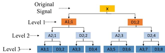
Fig. 4. Level-3 full wavelet packet transform. In  $A_{\alpha; \beta}$  and  $D_{\alpha; \beta}$ ,  $\alpha$  represents levels and  $\beta$  represents the index of the signal in level- $\alpha$ .
