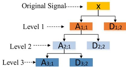
Fig. 3. 3-level wavelet transform. In  $A_{\alpha; \beta}$  and  $D_{\alpha; \beta}$ ,  $\alpha$  represents levels and  $\beta$  represents the index of the signal in level- $\alpha$ .
