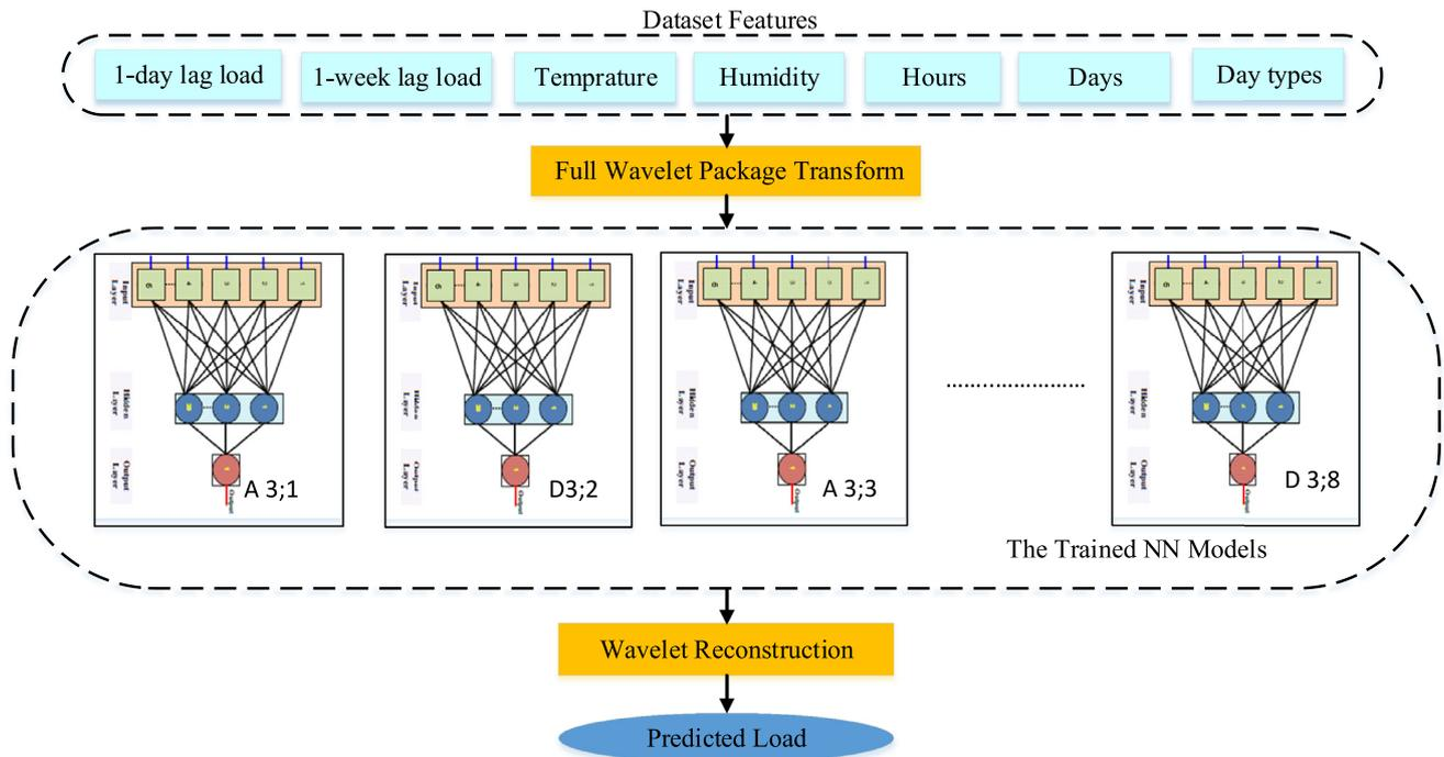
Fig. 5. The diagram of full wavelet neural network.
